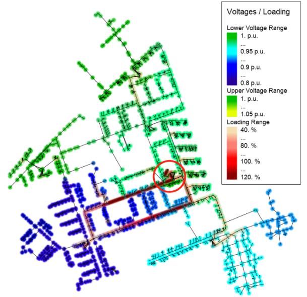
Fig. 1: Heat map showing the overloaded and under-voltage region in the suburban grid with 80 % EV penetration.
