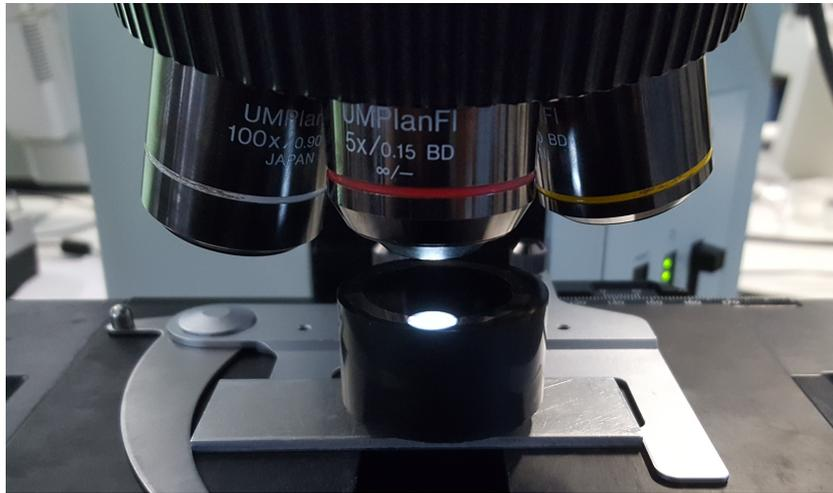
Figure 3.54: Optical microscope during analysis of a specimen
