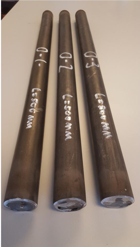
Figure 5.9: Cold-drawn carbon steel specimens
