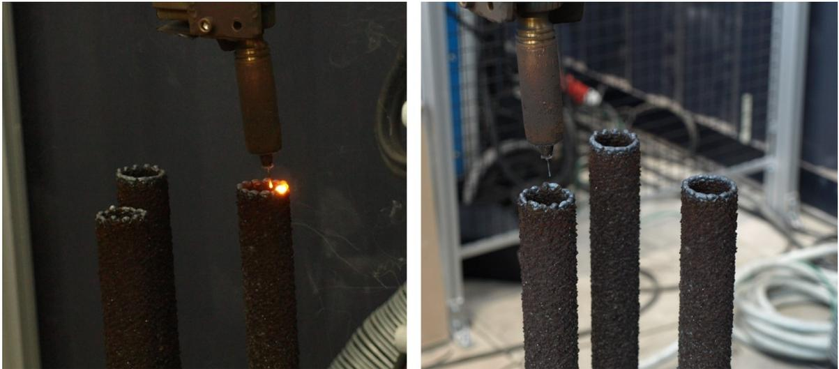
Figure 3.9: Printing according the 'Merlon strategy' with clearly visible its distinctive point welds
