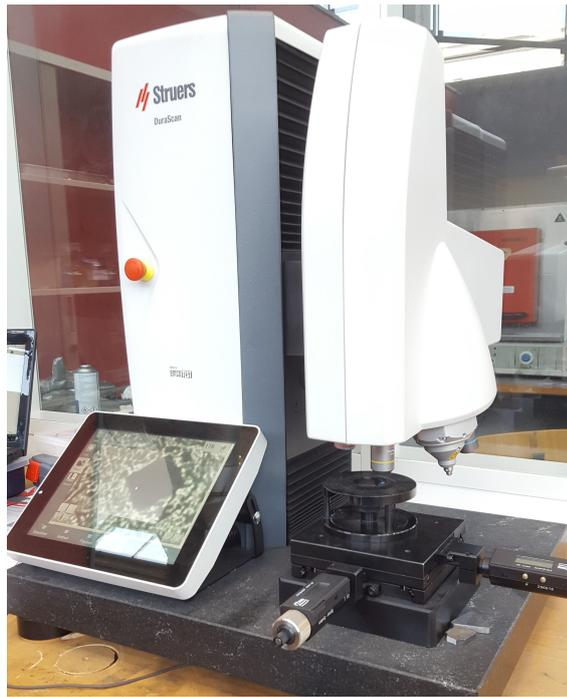
Figure 3.50: Struers Durascan G5 Hardness tester
