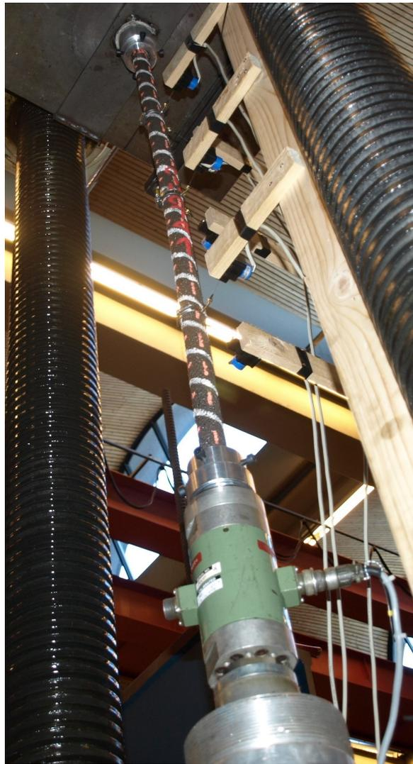
Figure 3.42: Buckling test on a printed column
