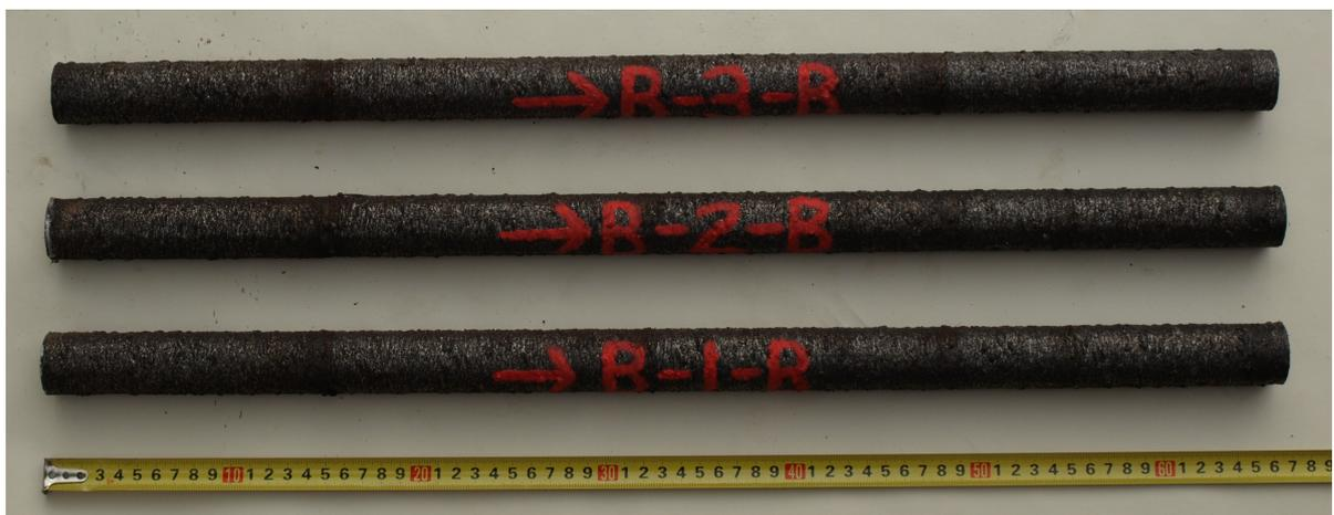
Figure C.5: Buckling and bending test specimens - 67 cm; continuous-strategy
