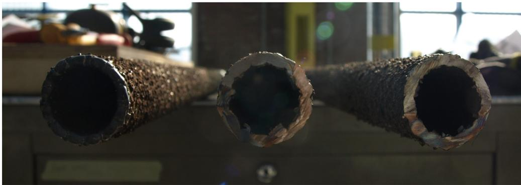
Figure 3.3: Column sections as cut from the welding plate with irregular cross-sections
