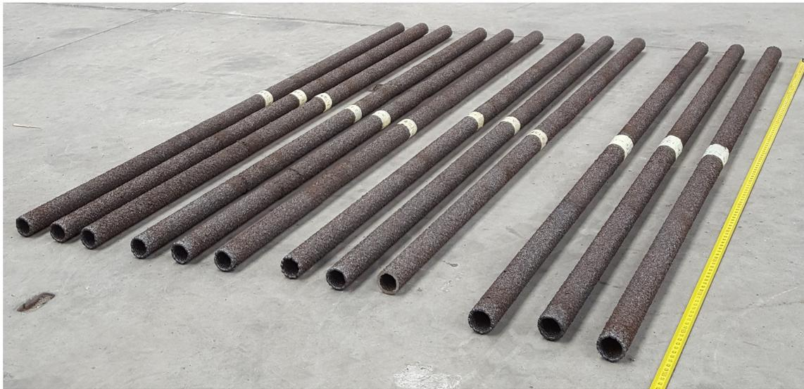
Figure 3.2: Tubular columns with a length of 1.30 metre as produced by MX3D's 3D-printing robot
