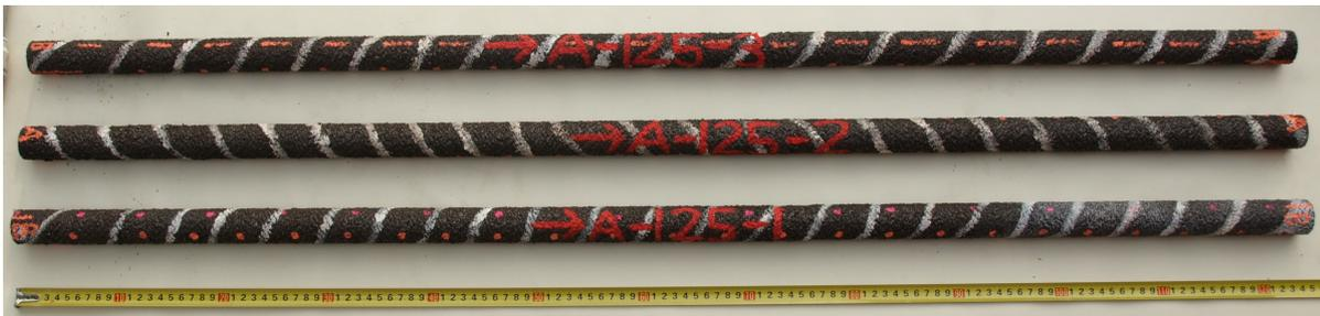
Figure C.1: Buckling test specimens - 125 cm
