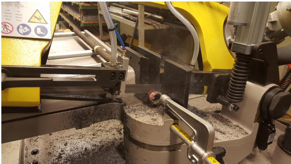
Figure 3.11: Columns are cut perpendicular by a belt-sawing machine
