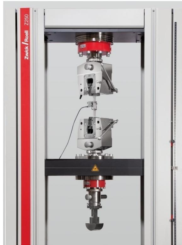
Figure 3.49: Zwick/Roell Z250 tensile test machine
