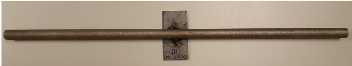
Figure 3.28: Round steel (20 mm) calibration specimen with welded plate to enable deflection measurement
