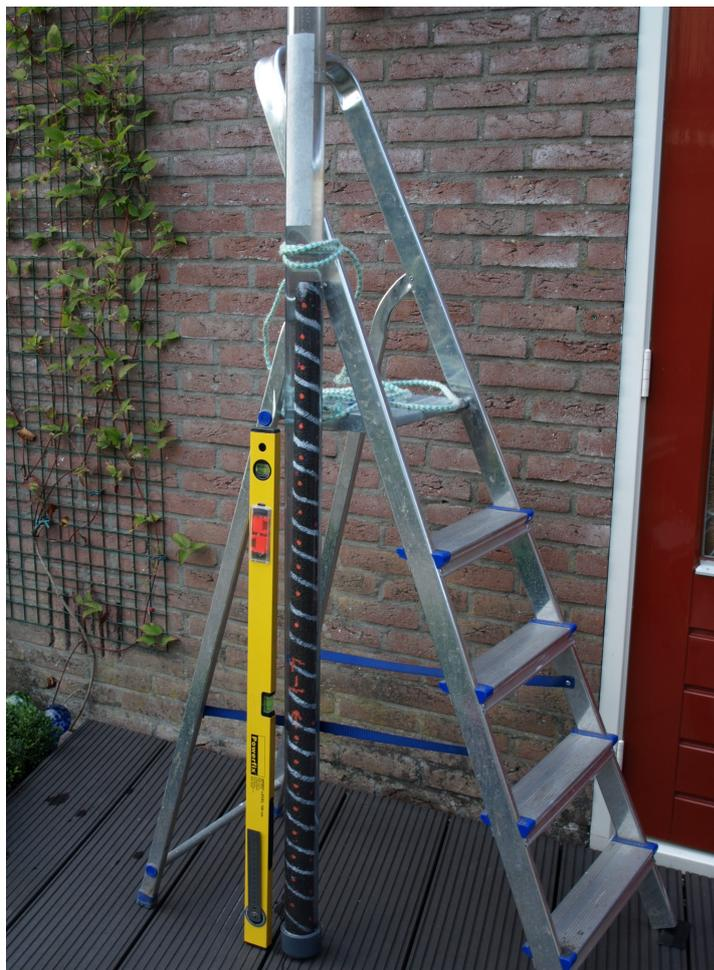
Figure 3.24: Set-up used to perform Archimedes' volume measurements
