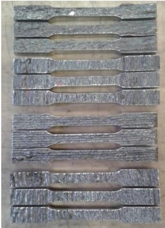
Figure 3.48: Milled tensile test specimens with A50-geometry
