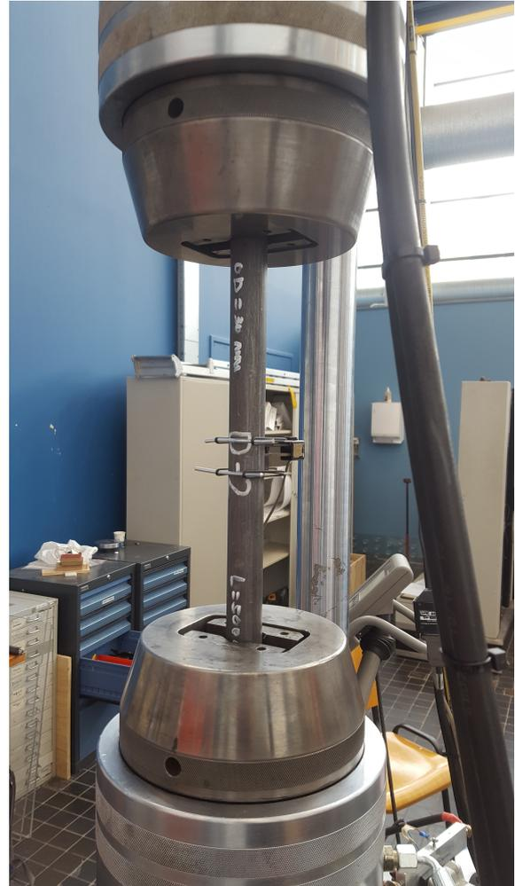
Figure 5.10: Tensile test set-up
