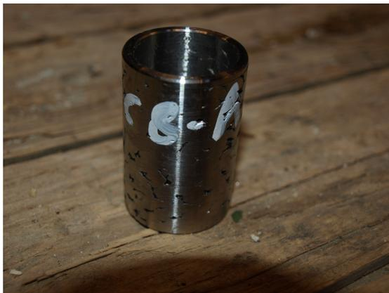
Figure 3.43: Milled dot-printed compression specimen
