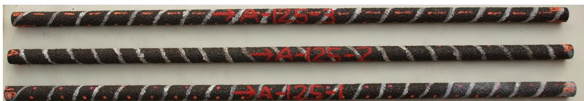
Figure 3.31: Buckling specimens with a length of 1250 mm including orange marks to depict the expected buckling direction
