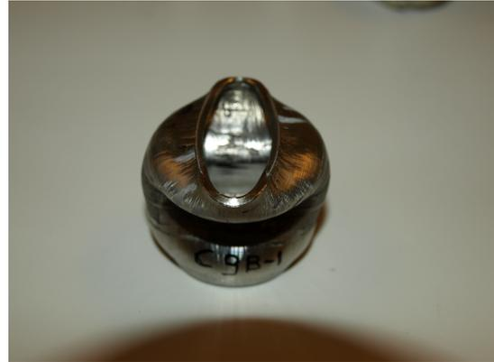
Figure 4.7: Specimen C9B after compression test
