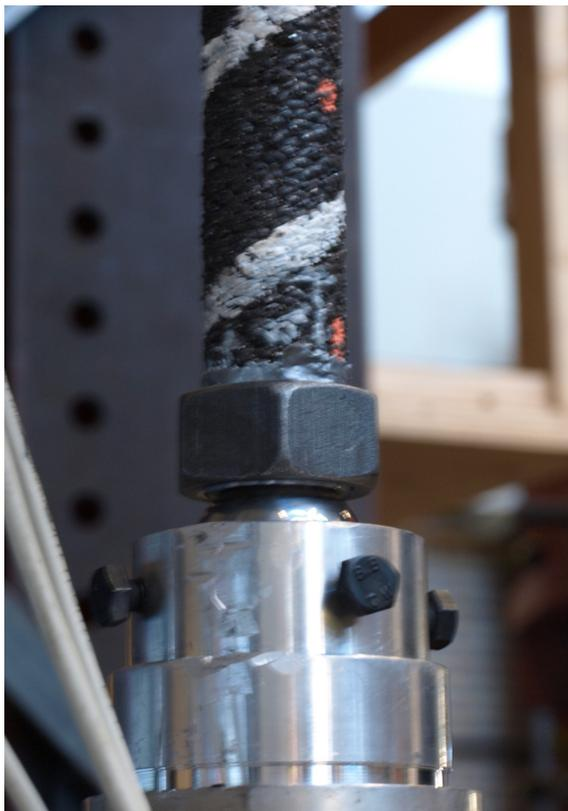
Figure 3.37: Column-end reinforcement with a bolt
