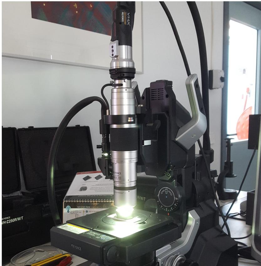
Figure 3.55: Microscope used to acquire composite images of the microstructure
