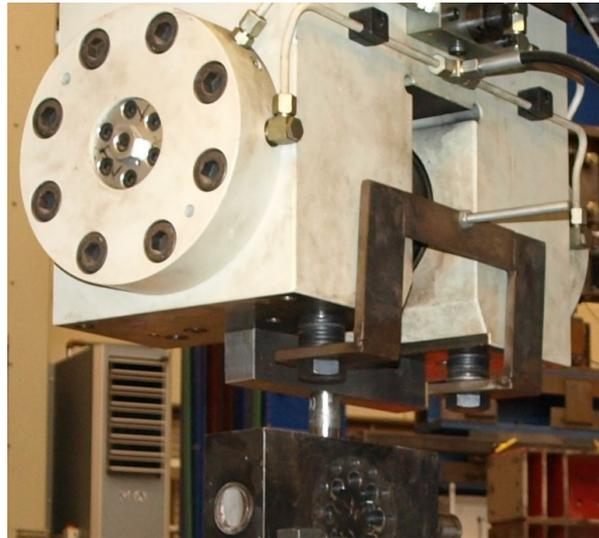
Figure 3.45: Compression test set-up
