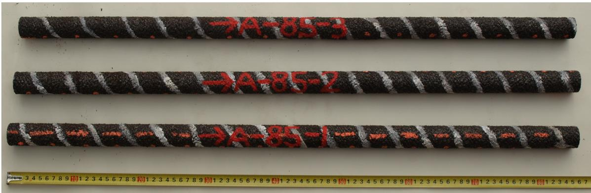
Figure C.2: Buckling test specimens - 85 cm
