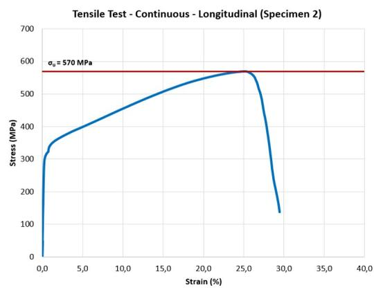
Figure C.60: Stress-strain: continuous - longitudinal (2)
