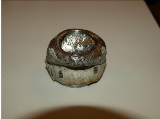
Figure 4.6: Specimen C8A after compression test
