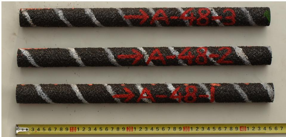
Figure C.3: Buckling test specimens - 48 cm
