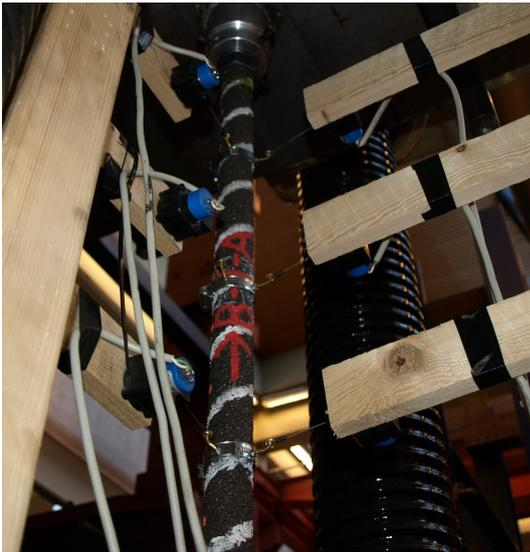
Figure 3.39: Location of linear displacement sensors
