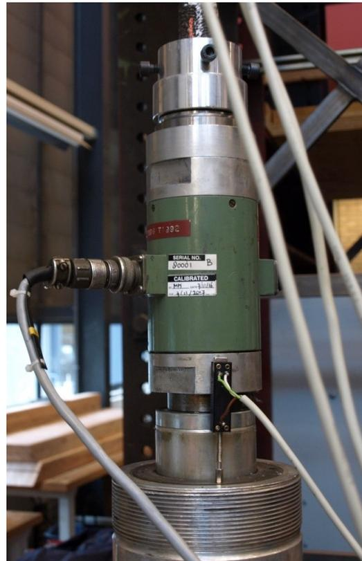
Figure 3.38: Pump, pressure box and displ. measurement
