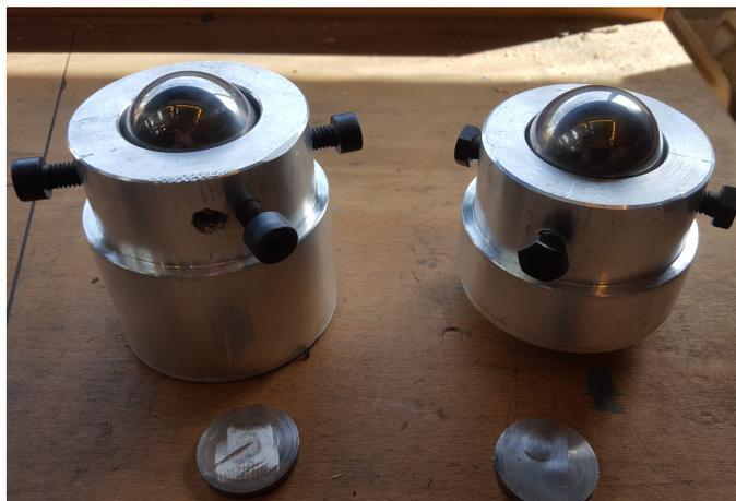
Figure 3.34: Ball bearings as they are used for buckling tests
