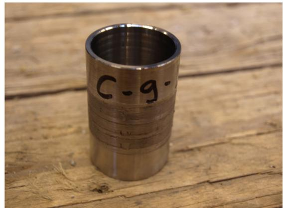
Figure 3.44: Milled continuously printed compression specimen
