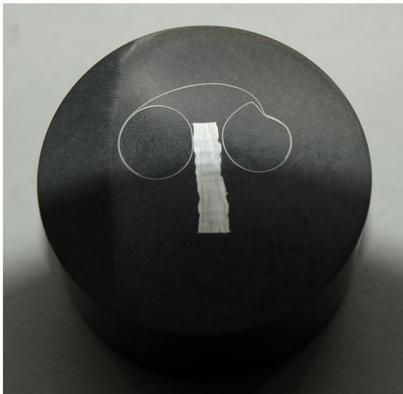
Figure 3.52: Longitudinal section prepared for micrography
