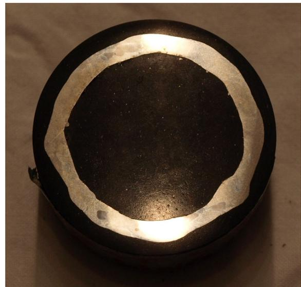
Figure 3.53: Transversal section prepared for micrography
