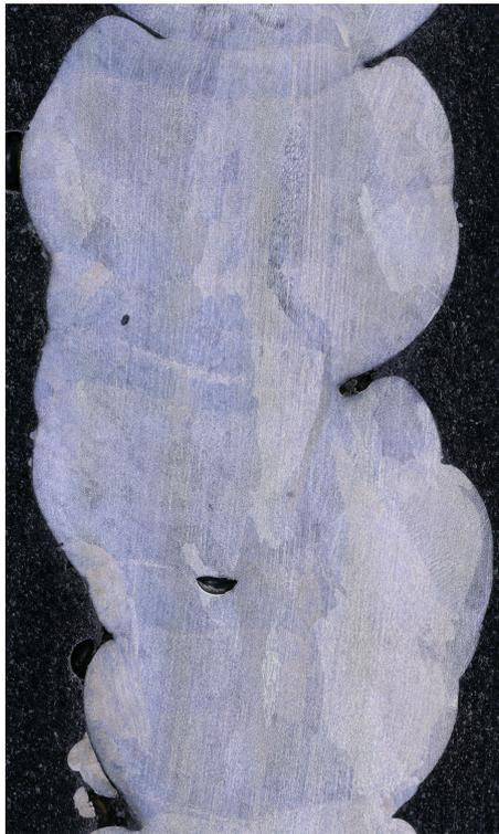
Figure 4.15: Longitudinal section dot-by-dot strategy
