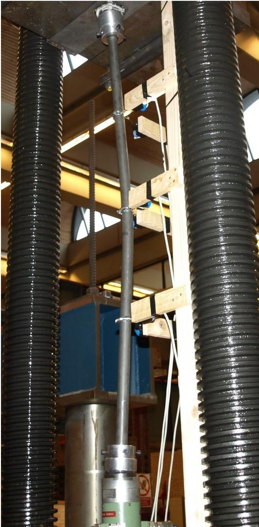
Figure 3.41: Buckling test on a cold-drawn tube
