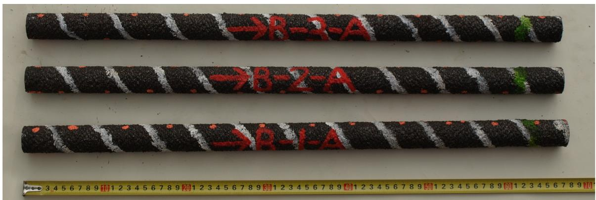
Figure C.4: Buckling and bending test specimens - 67 cm
