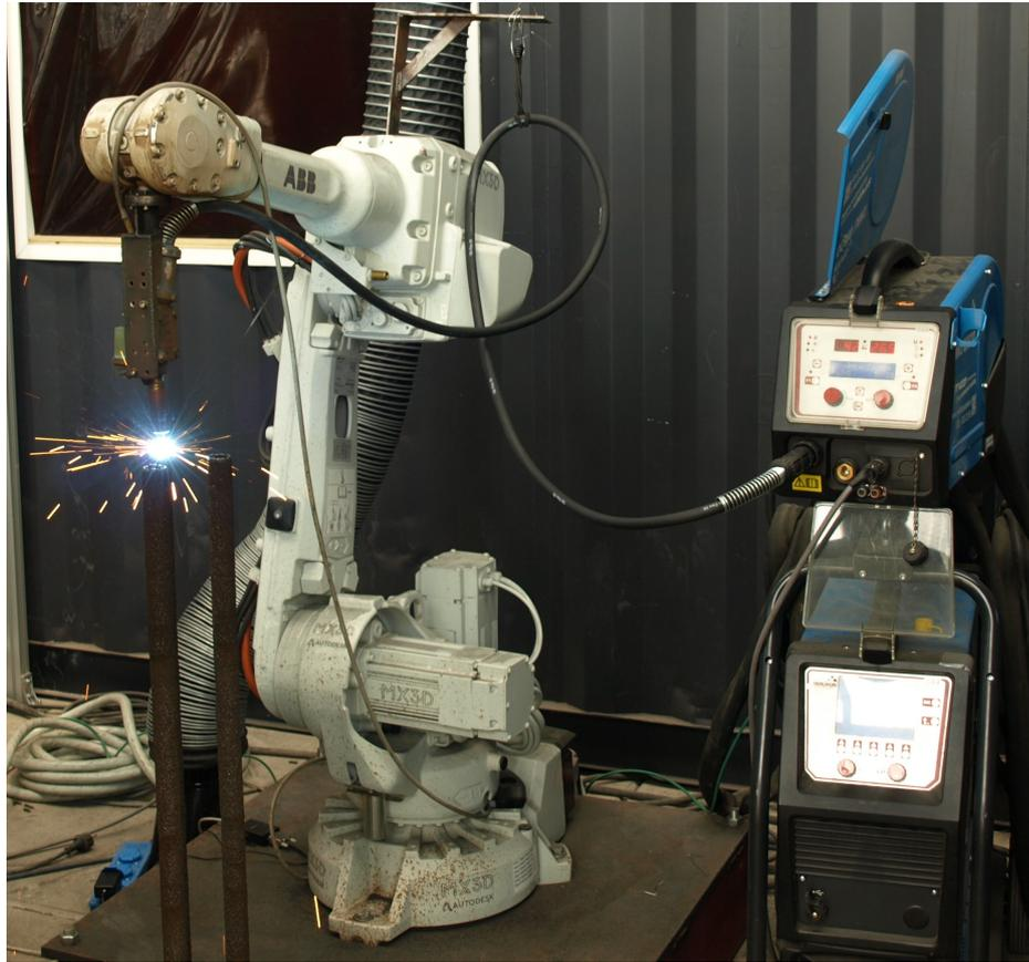
Figure 2.30: MX3D's printing set-up with multi-axis ABB IRB-5-2600 robot and Oerlikon Citowave 3 GMAW-system
