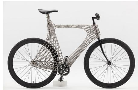
Figure 1.4: WAAM steel bike frame (MX3D/TU Delft)
