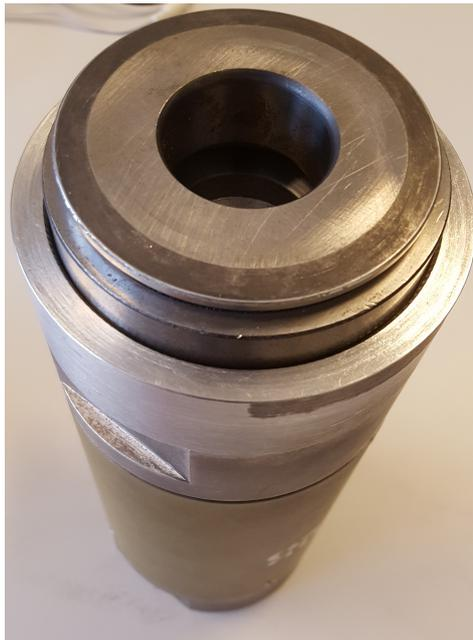
Figure 3.32: First test: spherical plain bearing
