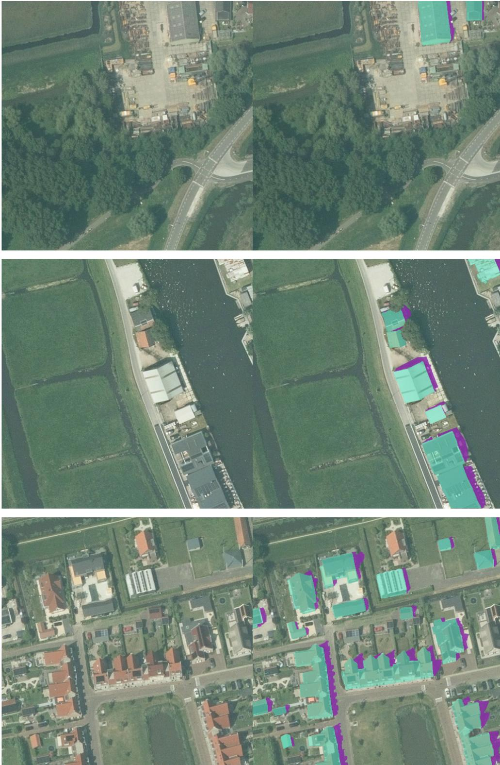
Figure G.1: Three images showcasing the original RGB on the left, with the manually annotated masks on the right. Purple for building shadows, teal for building footprints.
