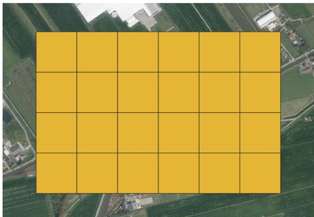
Figure D.2: During step 2, using the "Create Grid" option from the QGIS Toolbox, a 512x512 grid is overlaid. To do so, spacing was set to 512x0.25 (25cm resolution) to get 128x128 meter grid cells. From here, the underlying raster can be clipped by iterating over each polygon within the grid layer individually while outputting.
