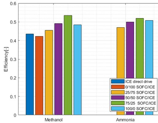
Figure 4.19: Efficiencies for different power configurations per fuel.
