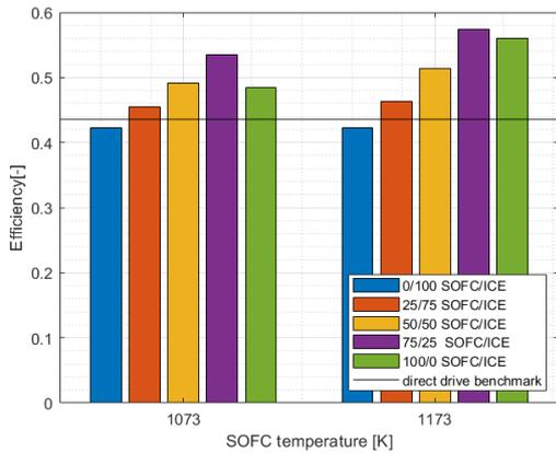
Figure E.8: Efficiencies for different power splits per SOFC operating temperature.
