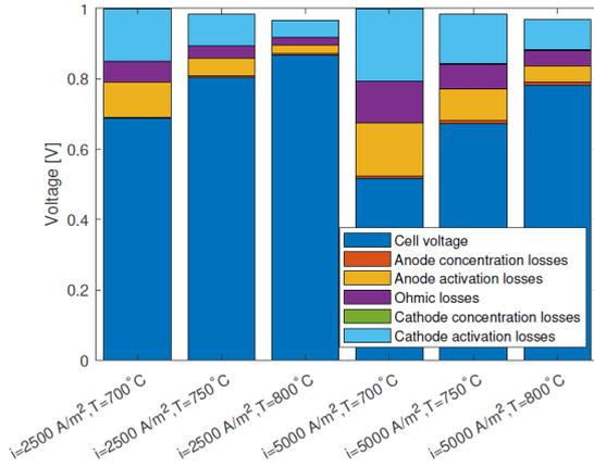
Figure 4.9: Cell voltages for different current densities and temperatures while running on ammonia by Koekkoek [44].
