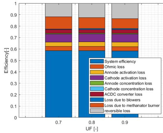
Figure 4.4: Different losses per UF.
