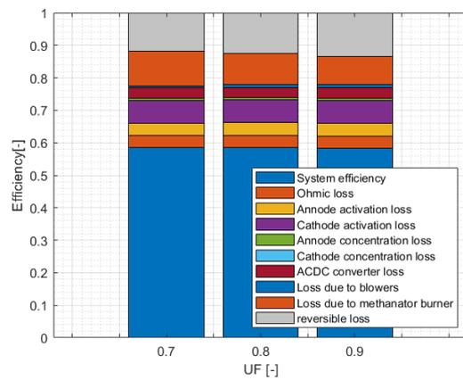
**Figure E.3:** Different losses per UF.
