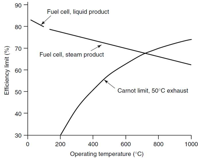
Figure 2.3: maximum efficiency of a hydrogen FC and heat engine [48].
