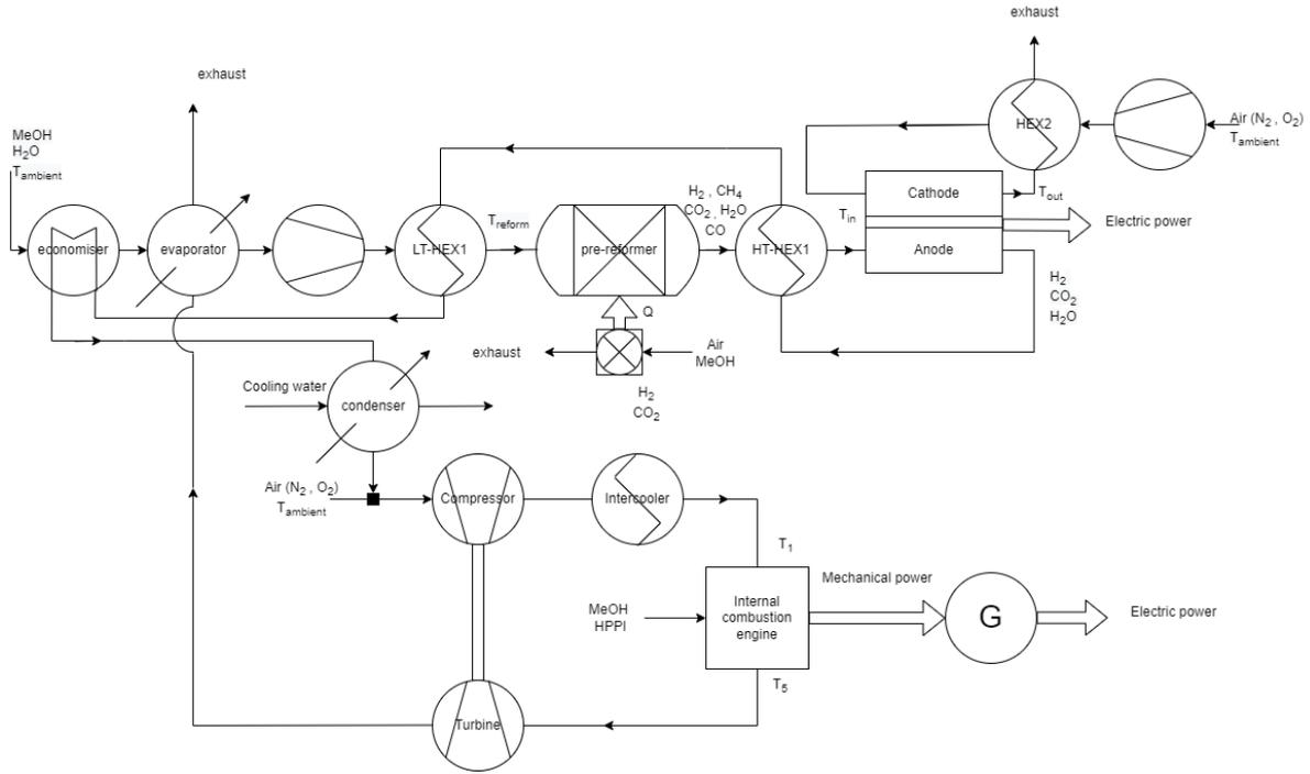
Figure E.1: Schematic representation of the combined SOFC-ICE cycle.
