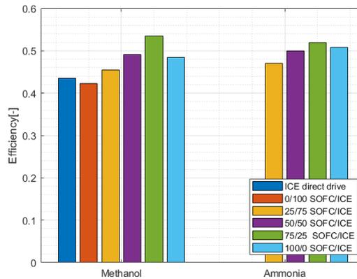
**Figure E.10:** Efficiencies for different power configurations per fuel.**Table E.3:** Data on the efficiency [%] from Figure E.10. Estimate given in *italic*.
