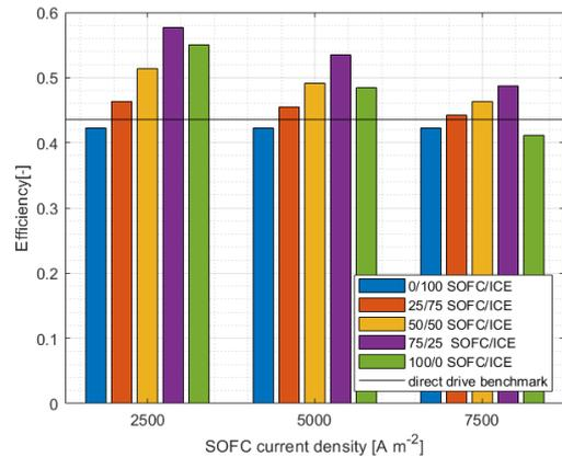
Figure E.9: Efficiencies for different power splits per SOFC current density.
