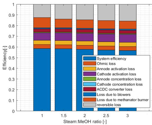
**Figure E.2:** Different losses per steam:methanol ratio.
