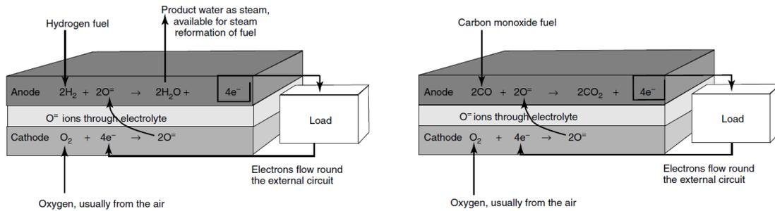
**Figure 2.2:** Schematic view of the reactions in an SOFC fuelled with hydrogen (first figure) or carbon monoxide (second figure) [48].
