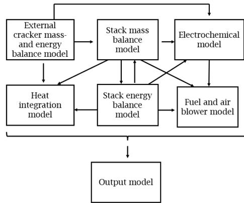
Figure 3.1: Block overview of the SOFC model proposed by Koekkoek [44].
