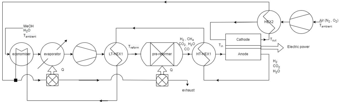
Figure 3.4: Layout of the SOFC plant including the heat integration.
