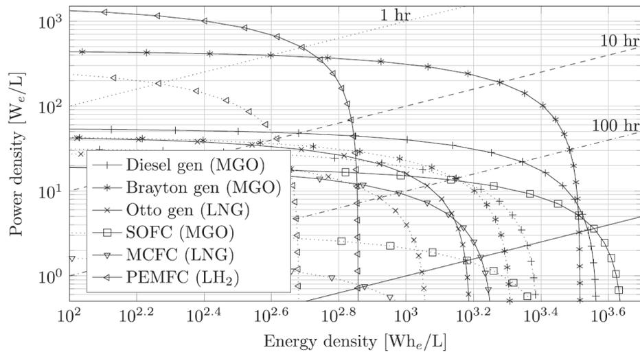
**Figure 2.4:** Power densities and energy densities for different drive systems and fuels. The dashed lines corresponds to the conservative estimates and the solid lines correspond to the upper estimates. [5]
