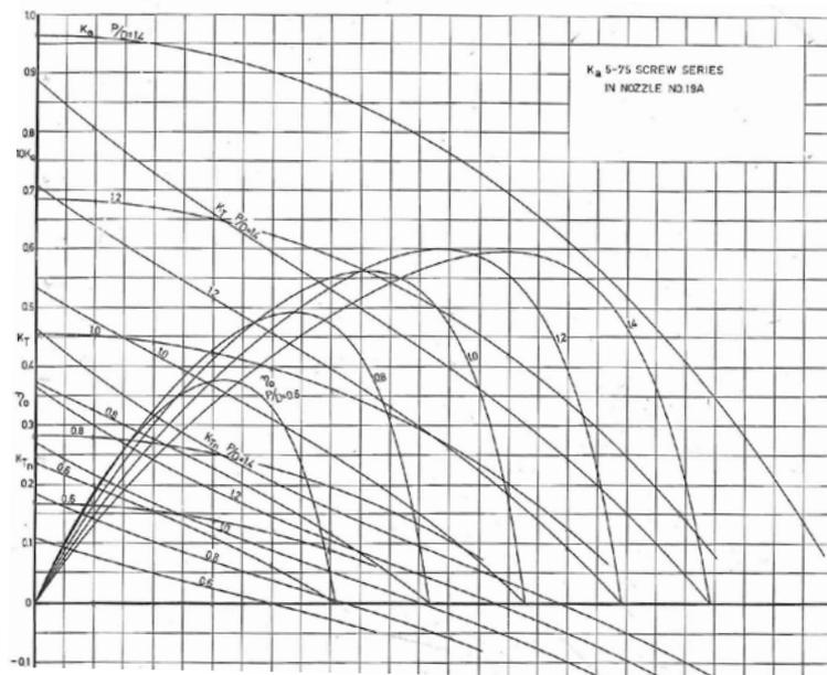
Figure 48: Open water curve at different pitch angles (KA 5-75 screw in NO.19A nozzle)
