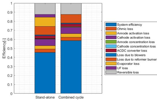
Figure E.6: Methanol-fuelled SOFC efficiency performance in standalone and combined cycle condition.
