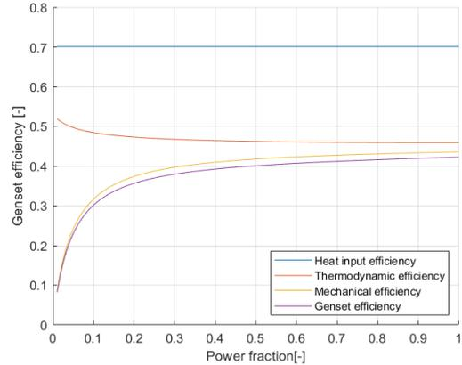
Figure E.7: Different efficiencies between 1% and 100% nominal power.
