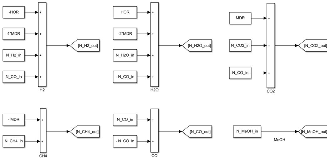
Figure 3.3: Schematic view of the mass balances per substance.
