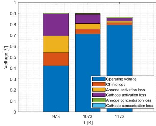
Figure 4.10: Cell voltages for different temperatures at a current density of  $5000 \text{ A} \cdot \text{m}^{-2}$  while running on MeOH.
