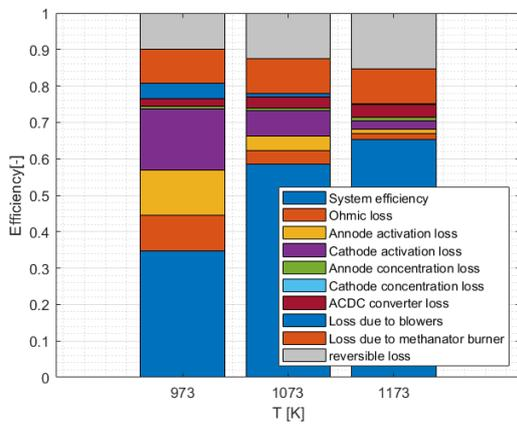
Figure 4.5: Different losses per T.
