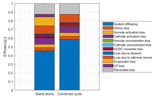
Figure 4.8: Methanol-fuelled SOFC efficiency performance in standalone and combined cycle condition.
