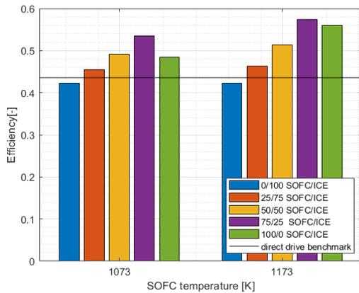
**Figure 4.17:** Efficiencies for different power splits per SOFC operating temperature.
