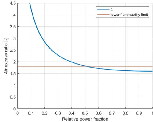
Figure 4.16: Air excess ratio and lower flammability limit [92].
