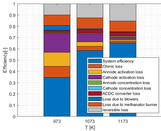
**Figure E.4:** Different losses per T.
