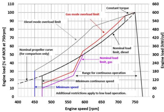
Figure 4.15: Engine envelope of the W31 [96].
