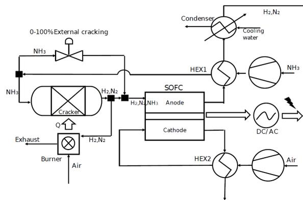
Figure 3.2: Layout of the SOFC model proposed by Koekkoek [44].
