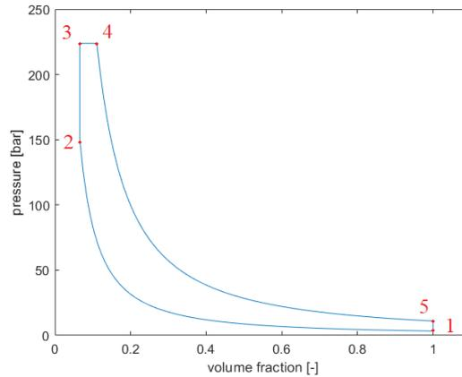
Figure 4.12: p-V diagram at nominal load with numbered Seiliger cycle stages.
