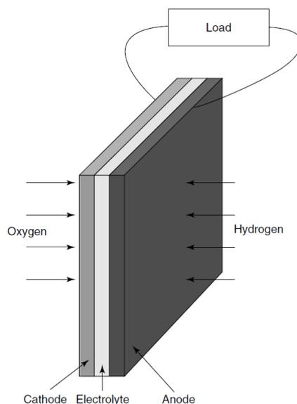
Figure 2.1: Schematic view of a single Cell [48].
