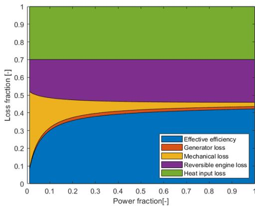
Figure 4.13: Different losses between 1% and 100% nominal power.
