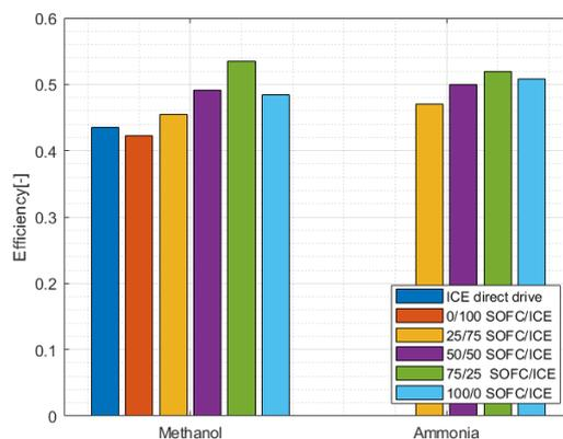
**Figure 5.1:** Figure 4.19 From Results : Efficiencies for different power configurations per fuel with (1)=MeOH and (2) = NH<sub>3</sub>.
