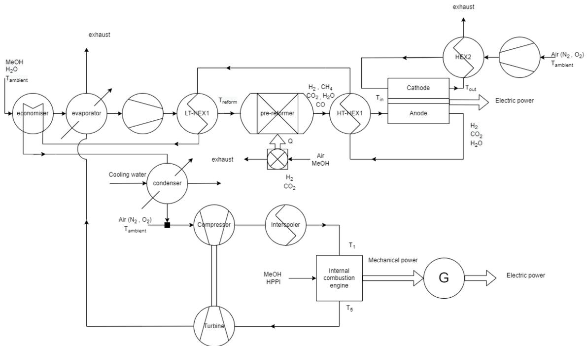
Figure 3.5: Schematic representation of the combined SOFC-ICE cycle.
