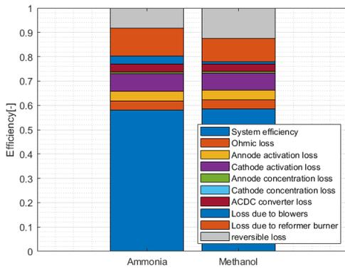
Figure 4.11: Different losses per fuel for standard conditions (Table 4.1).
