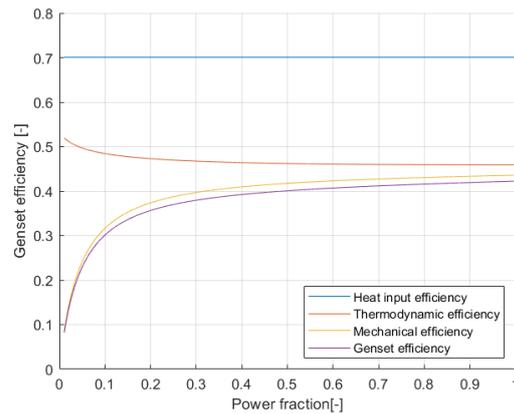
Figure 4.14: Different efficiencies between 1% and 100% nominal power.
