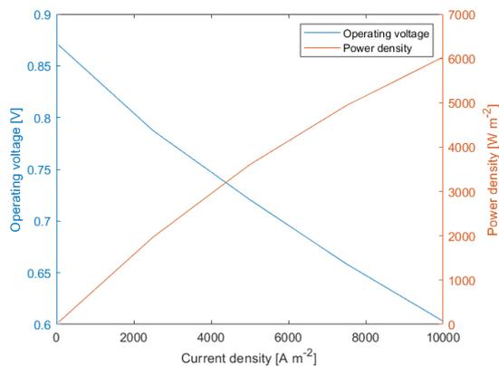
Figure 4.7: The operating voltage and power density of the cell against the current density.
