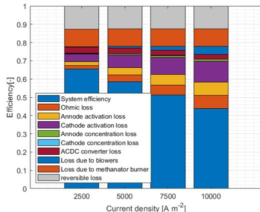
**Figure E.5:** Different losses per current density.
