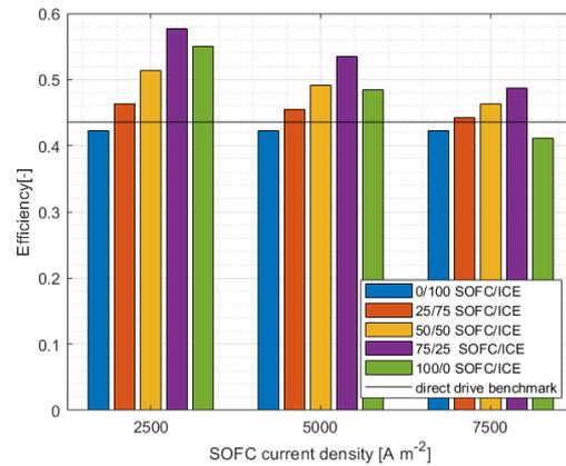
**Figure 4.18:** Efficiencies for different power splits per SOFC current density.
