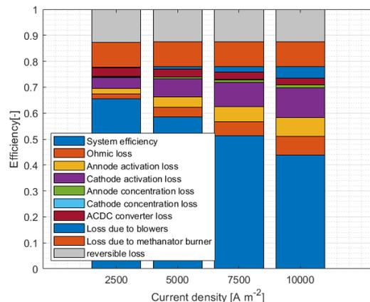
Figure 4.6: Different losses per current density.
