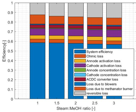
Figure 4.3: Different losses per steam:methanol ratio.
