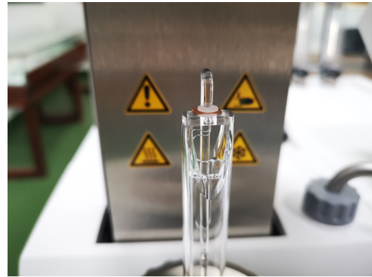
(b) Copper sample mounted on TMA equipment
