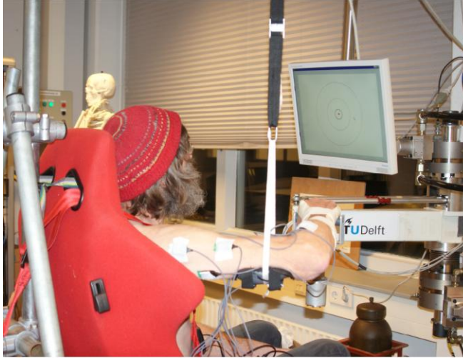
Figure 1. Experimental setup. The two joint manipulator was used to apply continuous force perturbations in two directions ( f_x and f_y ) onto the subjects hand. The manipulator acted as a mass-spring-damper system. The subjects arm was held in horizontal position by a rope mounted from the ceiling and the wrist joint was immobilized by a cuff fitted on the lower arm. The subjects were asked to perform three tasks.
