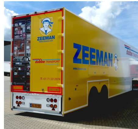
(b) Double-deck trailer for the transportation of standardised RCs (Burgersgroup B.V., 2018)
