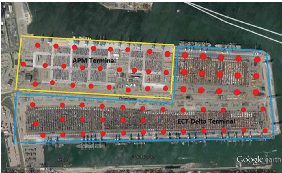
Figure 3: Lighting configuration of ECT and APM Rotterdam.
