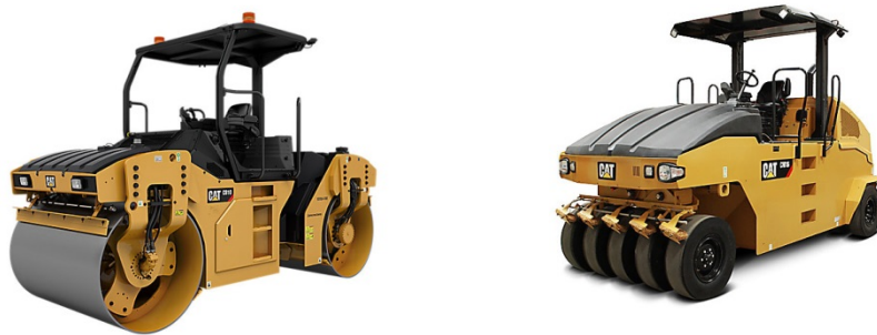
Figure 5.3 Static/vibratory roller (l) and Pneumatic roller (r) for compaction [58]
