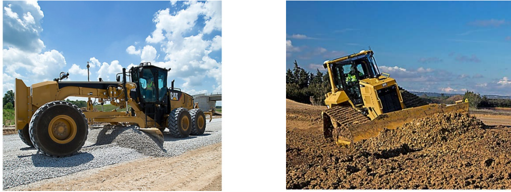
Figure 5.1 Motor grader (l) and Dozer (r) for pavement site preparation [58]
