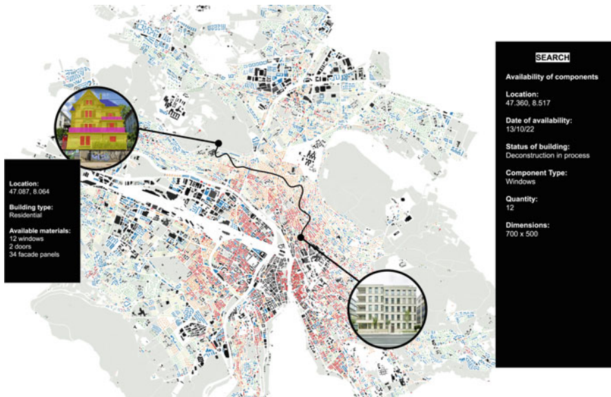
Fig. 4.2 Visualisation of database with insights on materials and components in supply project (or donor project) derived using CV that can be used for new construction projects (image from Raghu, D., adapted from De Wolf et al., 2023)
