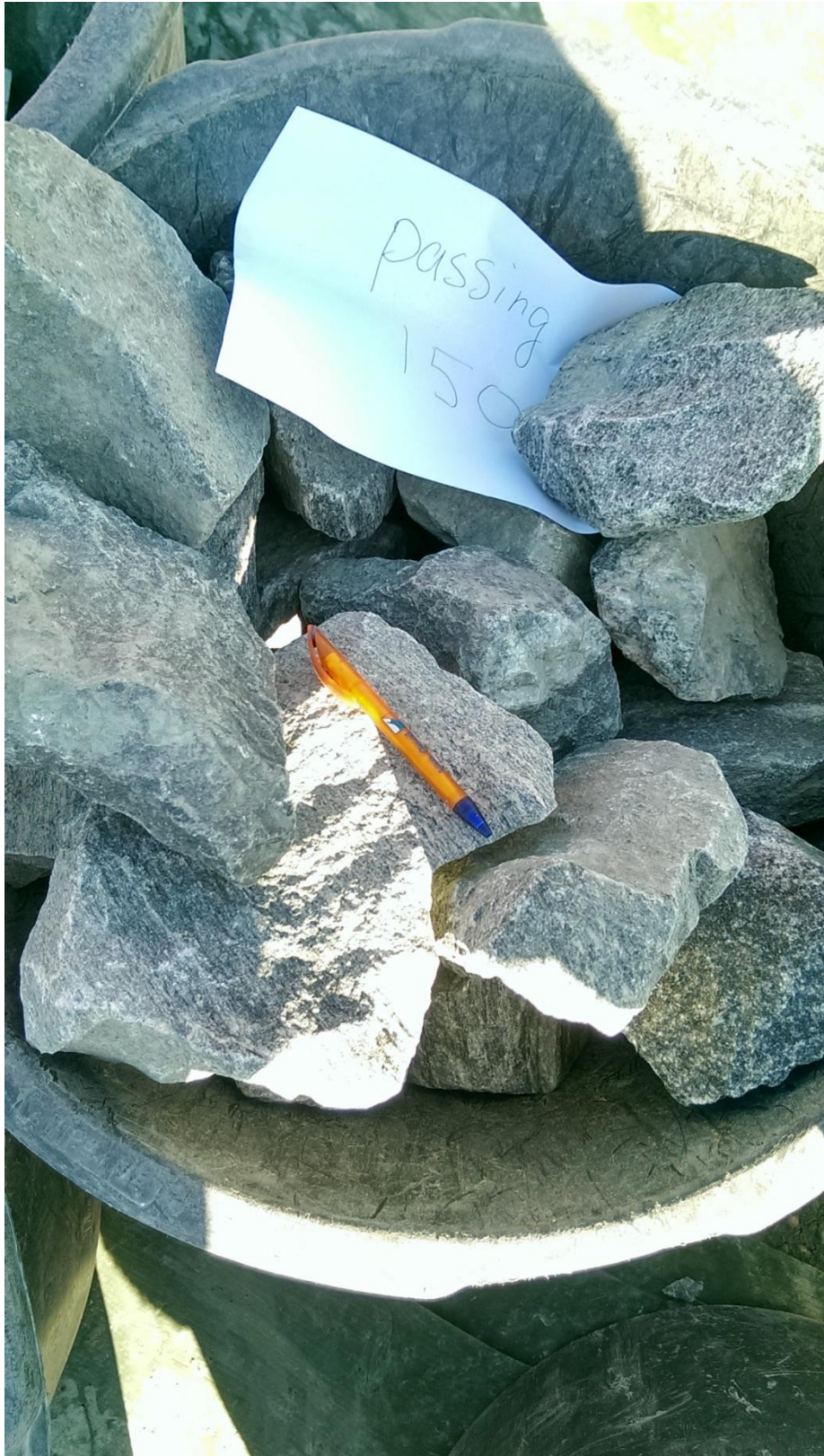
Figure B-22 - 125-150 mm, sample C, grading 5+ inch
