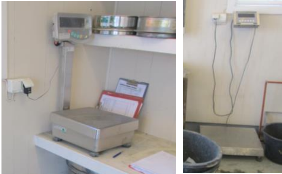
Figure A.2-6 left: low capacity balance, right: high capacity balance
