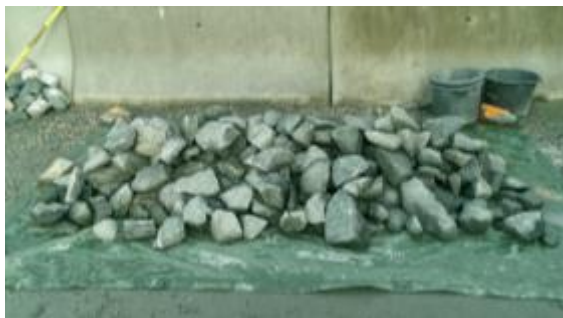
Figure A.2-1 sample reduction on 5+ material (test 2-3)
