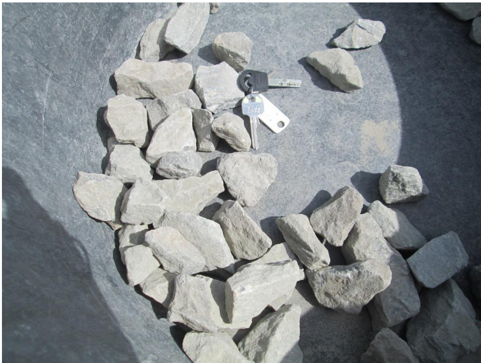
Figure B-5 - 31.5-45 mm, sample E, grading 2-8 inch
