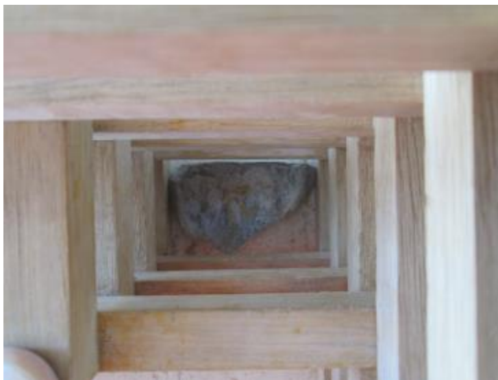
Figure A.1-3 measuring the smallest enclosing rectanguloid of a rock
