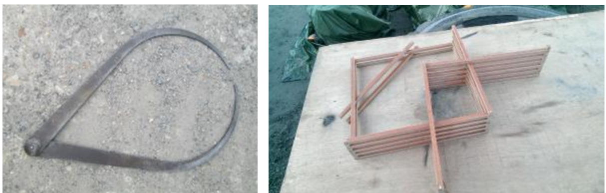
Figure A.2-5 left: calliper, right: blockiness-meter
