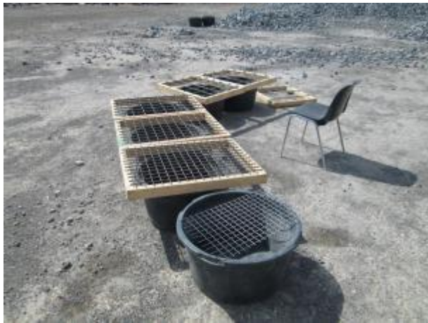
Figure A.1-4 sieving setup
