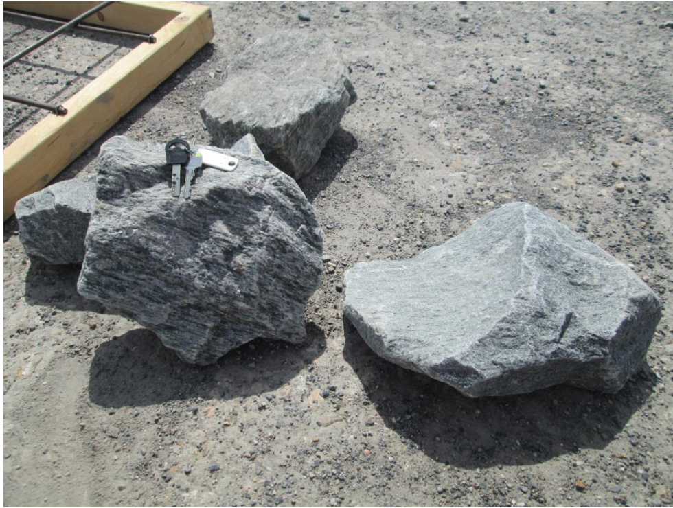
Figure B-10 - 180-250 mm sample E, grading 2-8 inch
