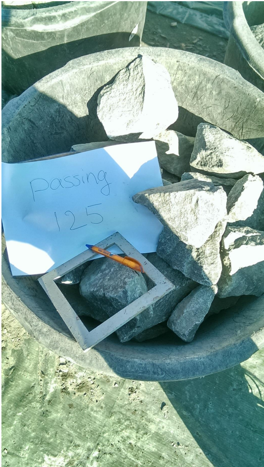
Figure B-21 - 90-125 mm, sample C, grading 5+ inch
