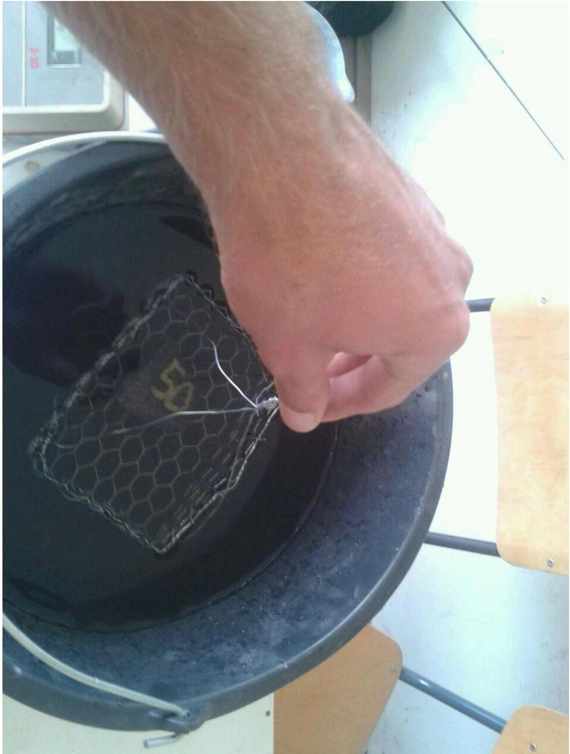
Figure B-12 - container to submerge rocks
