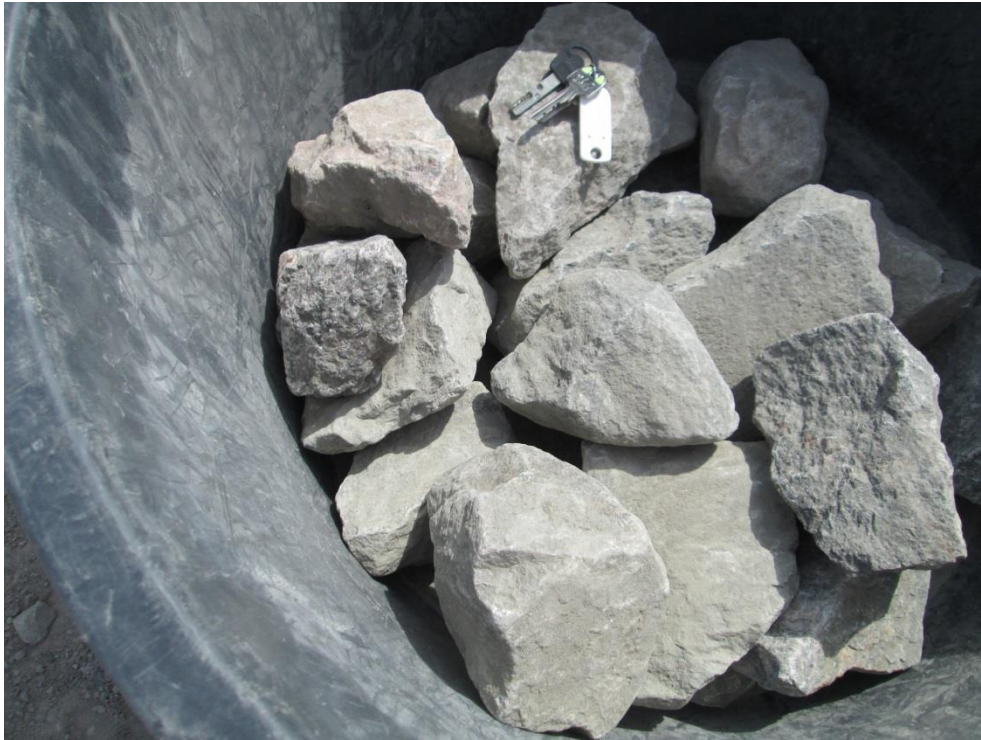
Figure B-8 - 90-125 mm, sample E, grading 2-8 inch
