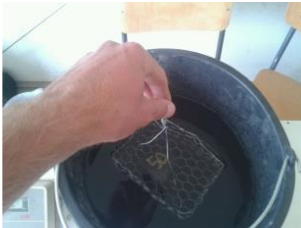
Figure A.1-2 submersion of a rock
