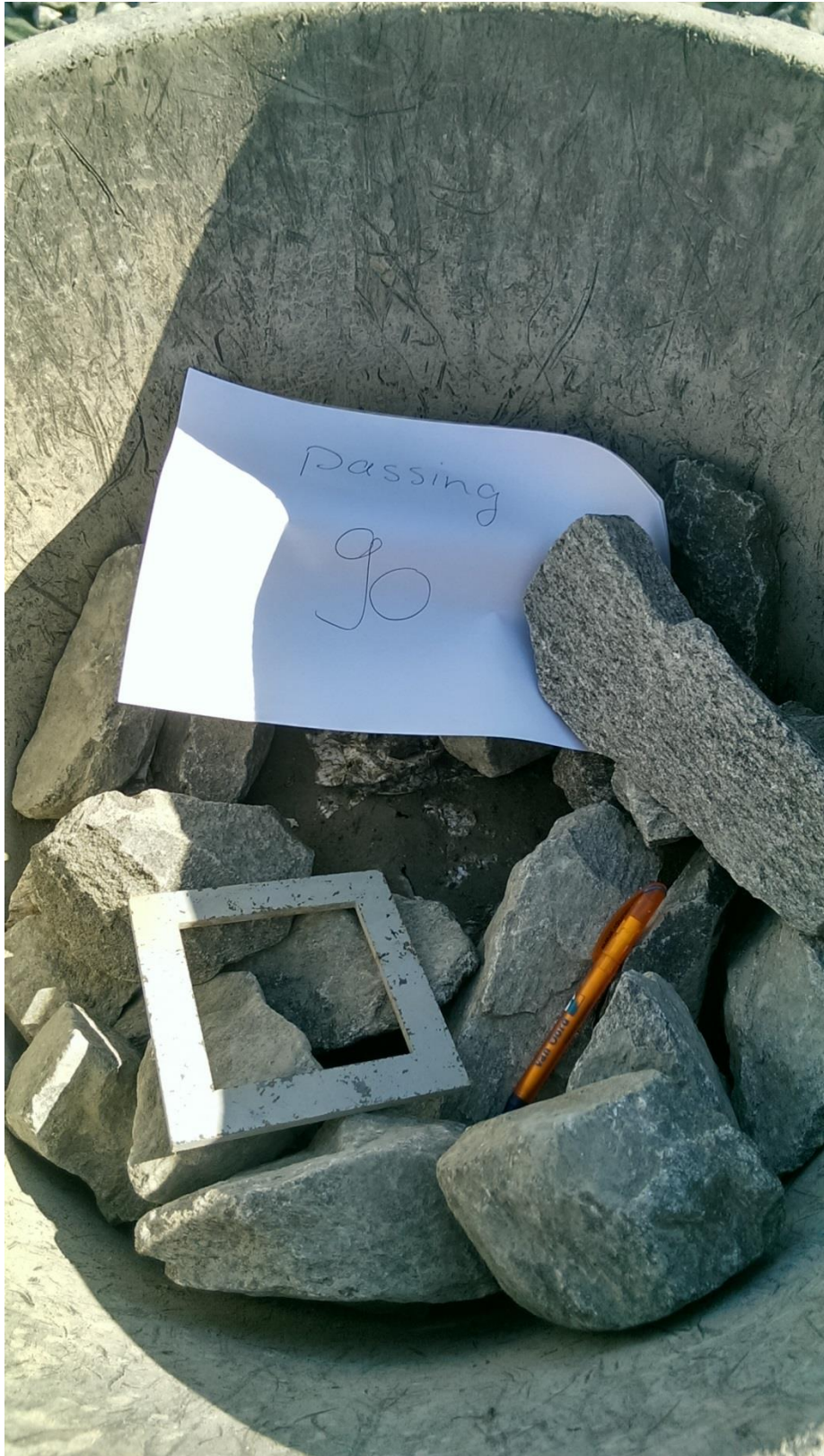
Figure B-20 - 63-90 mm, sample C, grading 5+ inch
