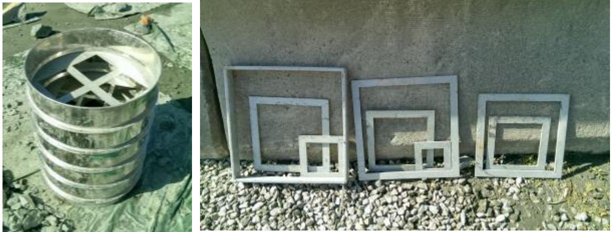
Figure A.2-4 left: drum sieve setup, right: steel plate sieves
