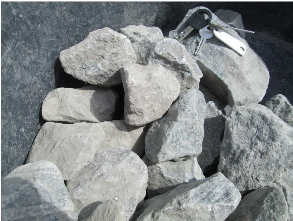
Figure B-7 - 63-90 mm, sample E, grading 2-8 inch
