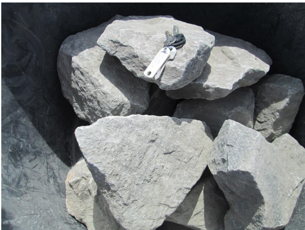
Figure B-9 - 125-180 mm, sample E, grading 2-8 inch
