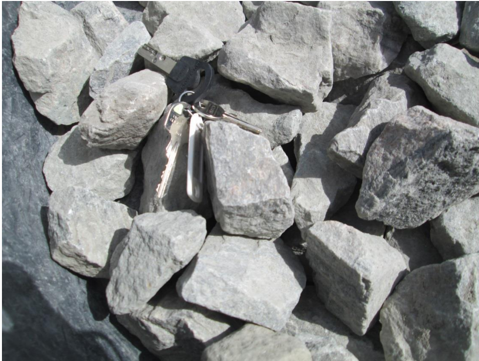
Figure B-6 - 45-63 mm, sample E, grading 2-8 inch
