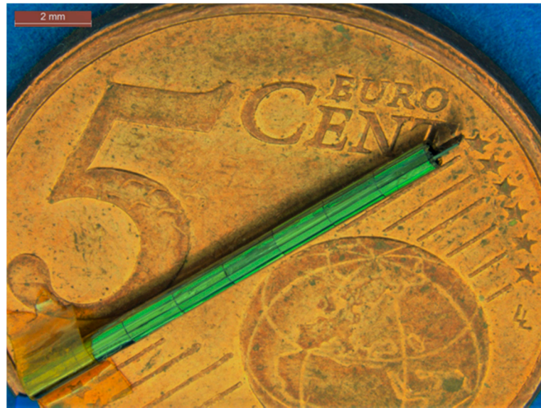
Figure 10. DBS demonstrator wrapped into a cylindrical probe with a length of 18 mm and a diameter of 1.2 \mu\text{m} .
