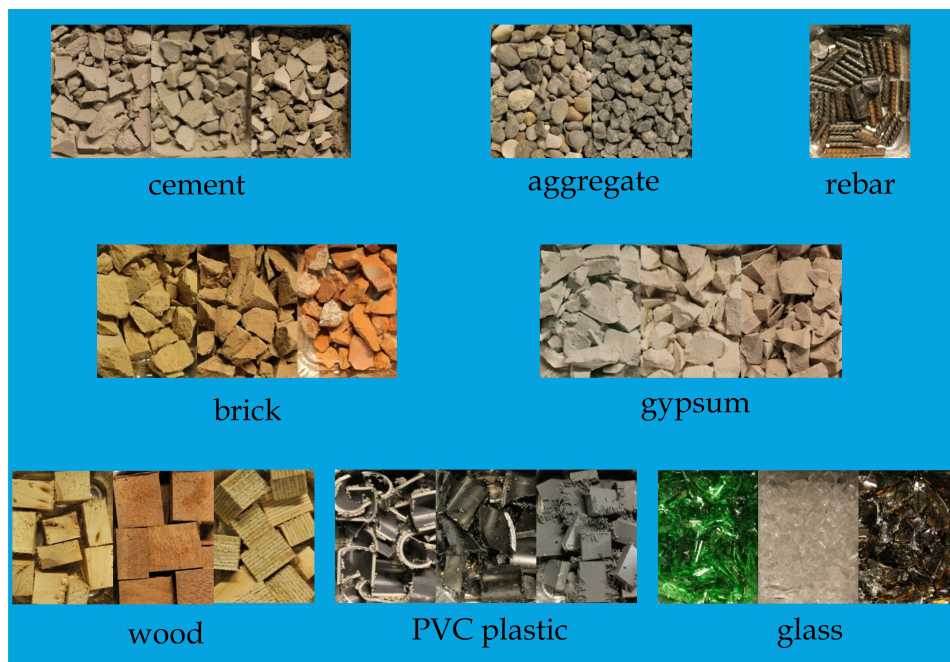
Figure 6.8: Eight waste materials and 21 selected types from a stream of demolition concrete.
