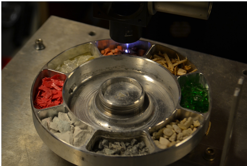
Figure 6.9: Granular materials mounted on a rotating plate. Laser-induced plasma is visible on a brick particle.
