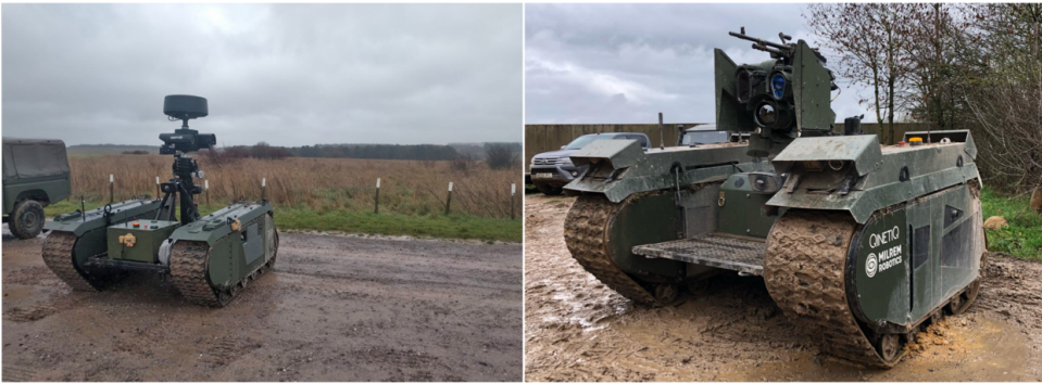
Figure 1.1.: THemis unmanned ground vehicles, part of the RAS unit
