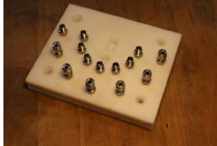
Figure 17. Backbone prototype of Team ZEF1, CNC-milled POM, bolts mounting the plates to each other miss in the photograph taken
