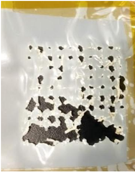
Figure 4.3: PEEK extrusion on a 0.05mm thick PEEK film, with the build platform at room temperature
