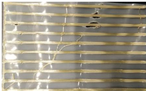
Figure 4.5: Extruded PEEK strips on a 0.05 mm thick film
