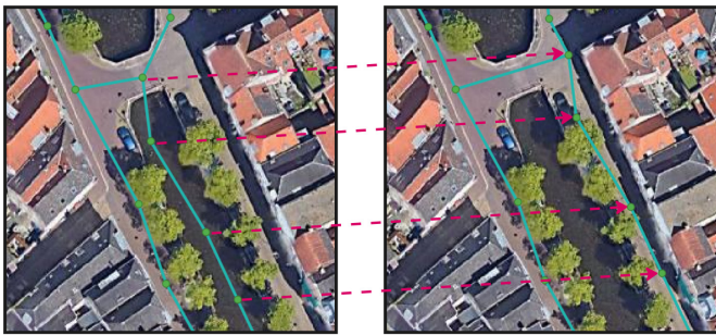
Fig. 5: Manual graph adjustment using our QGIS [34] plugin. Some of the nodes (green) are wrongly placed in a canal, but can be easily moved with one operation by a human annotator. The edges (blue) are automatically adjusted by the plugin.
