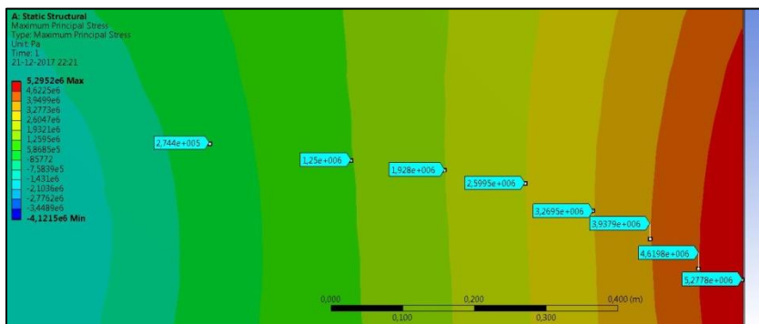
Figure 46: Tensile stresses in the ANSYS model used for determining forces
