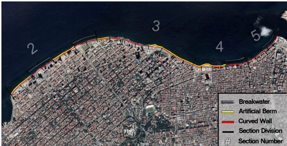
Figure 53: Overview solution coastal defence system Malecón
