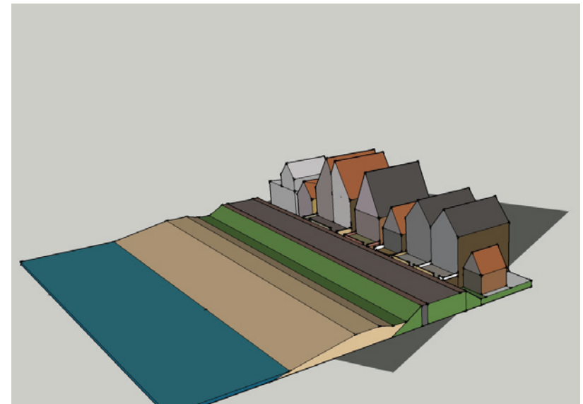
New Situation: new dike in front of the existing one. creating a 'vooroeverdijk'
