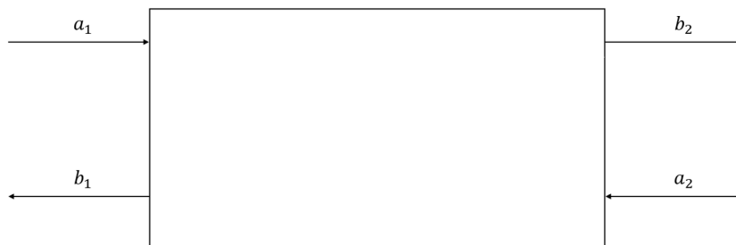
Figure 1.1: Illustration of a tube as a two-port network.
