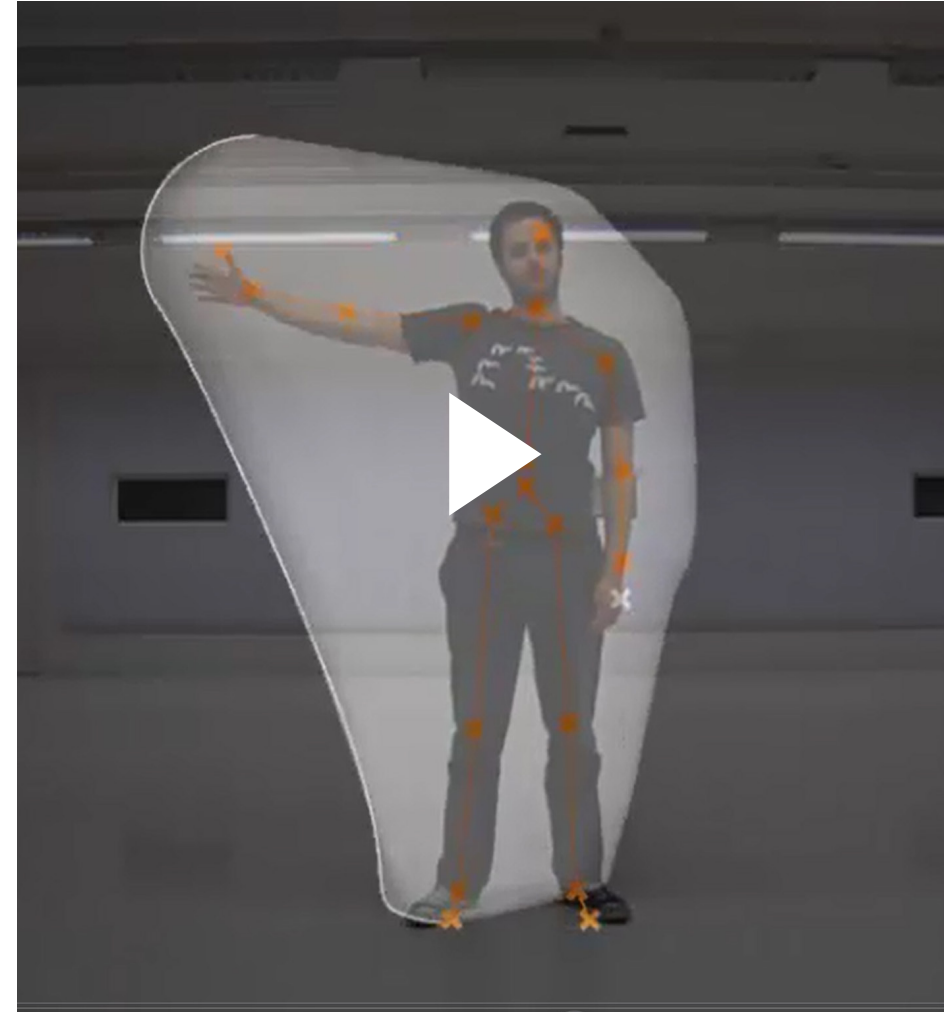
beginning to define a 3-dimensional space of occupancy around the skeleton. Every posture thus has a space associated to it.
