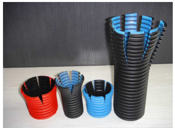
Figure 78. Corugated HDPE produced using a combination of pipe extrusion and blowmoulding.
