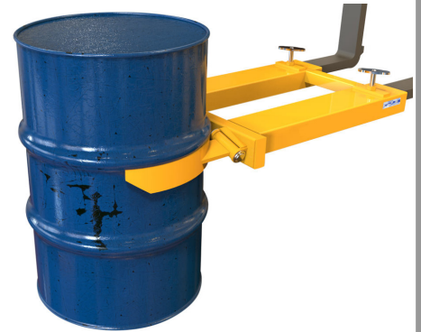
"Hugger": Arms at two sides surround the body of the drum. The rings of the drum prevent it from slipping down.
