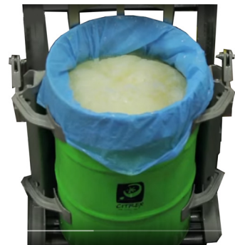
To empty the content the drum, it is placed on the "frame" of a tilting device and clamped in place, then tipped upside down.
