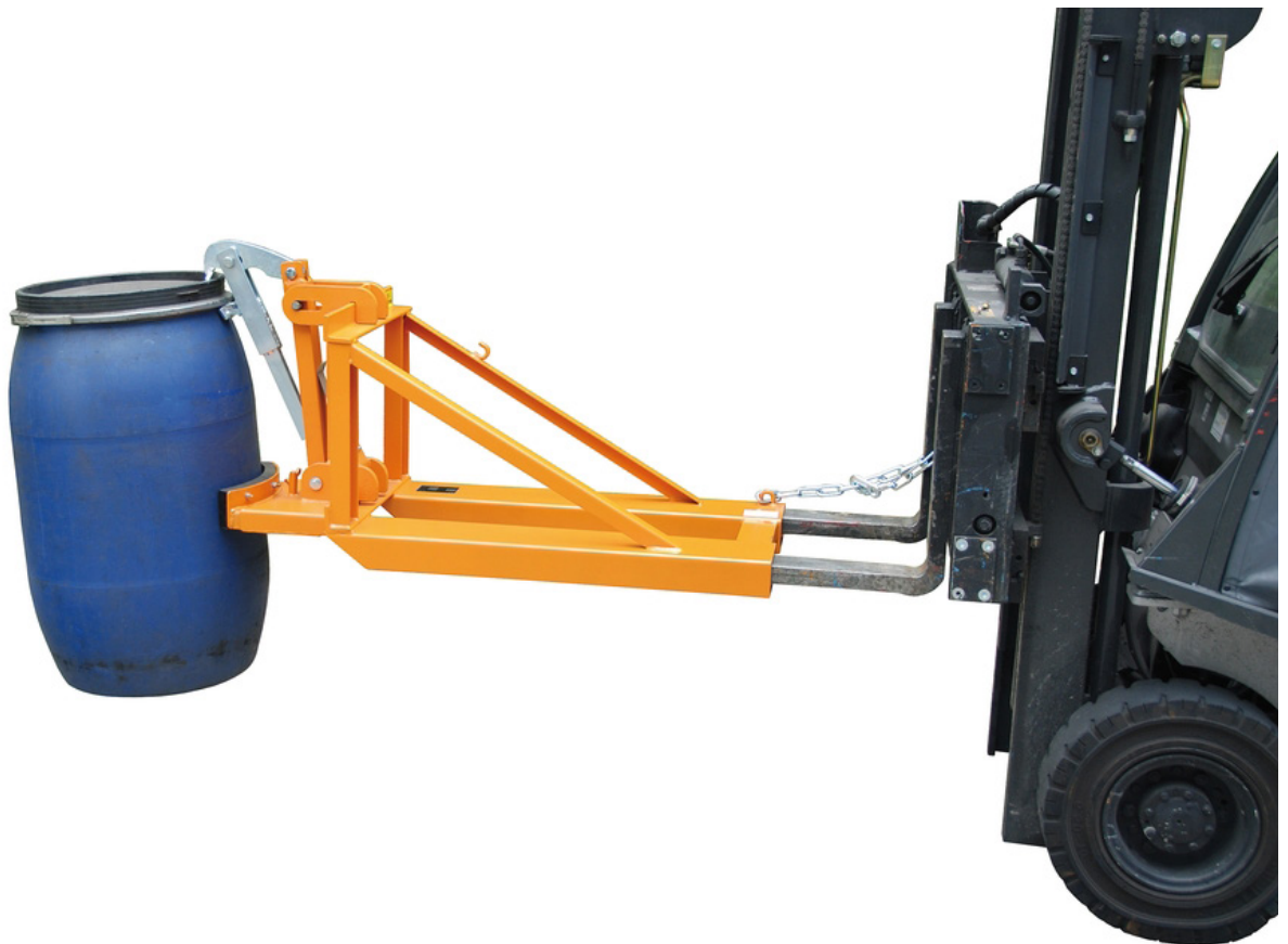
Figure 25. A forklift with a "pincher" tool (ELE, 2017)
