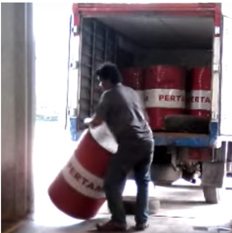
Rolled vertically, dropped out of a truck on an old tire
