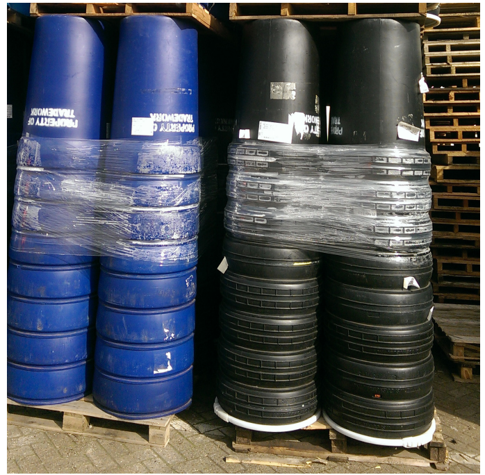
Figure 74. Empty N55 drums nested. 4*8=32 per pallet
