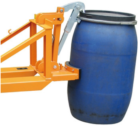
Forklift "Pincher": The "eagle claws" clasp hold of the rim of the drum and a support pushes against the body.
