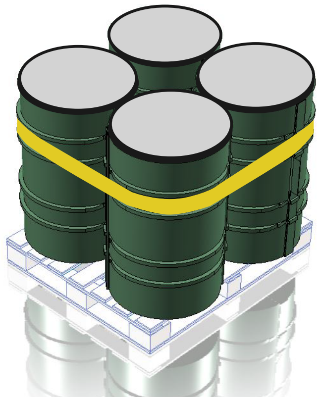
Figure 106. Four new drum on a 1.000 * 1.200 mm pallet. Strapped together (yellow band) for extra support.
