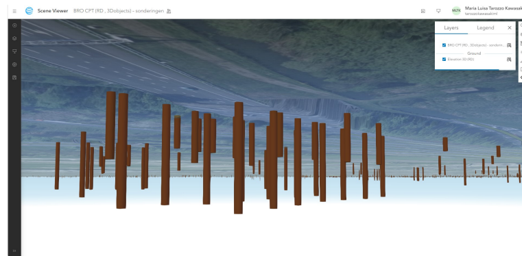
Figure 4.7: CPT boreholes visualized using 3D BRO webservice
