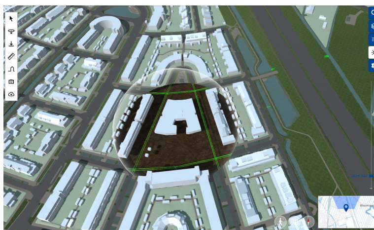
Figure 4.5: Subsurface congestion visualized using 3D Utrecht webservice
