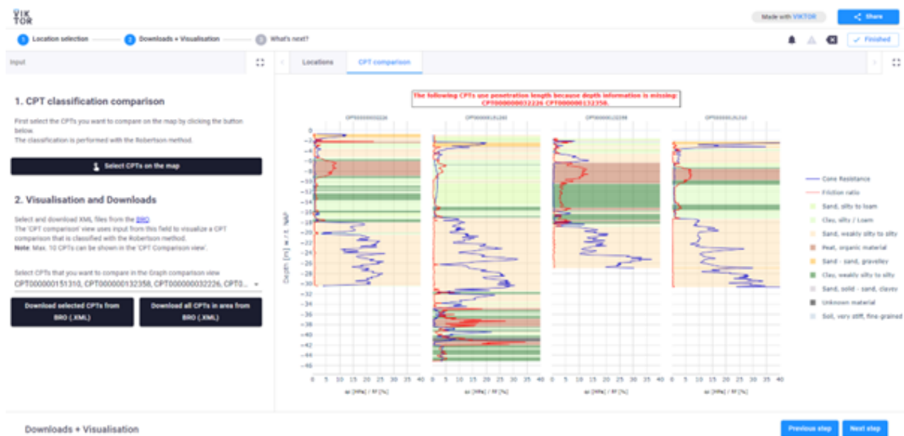
Figure 10.1: Visualization of CPT data classification using the webservice
