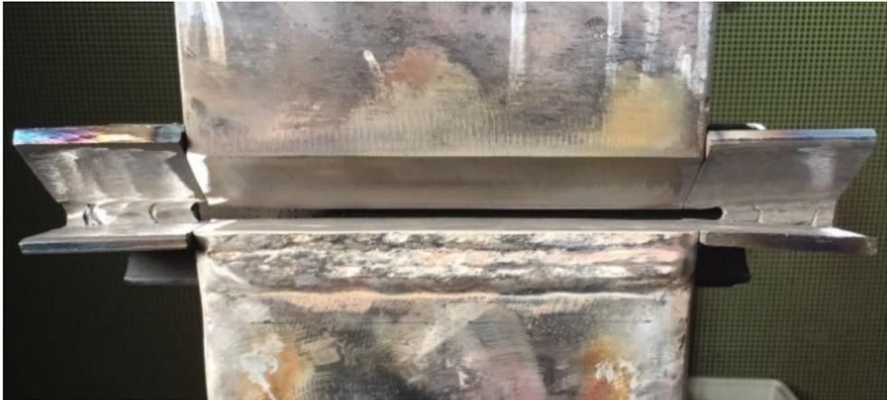
*Figure 5.18 Temporary plates for the repair of the edge cracks.*
