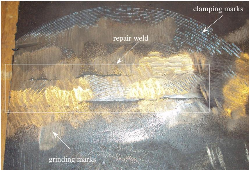
*Figure 3.16 Repair weld in the base material and grinding marks on the plate surface.*
