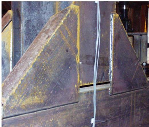
*Figure 4.19 Test specimens with complex attachment brackets [Dexter et al., 2003].*
