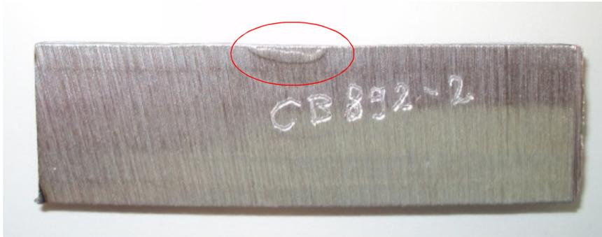
*Figure 3.11 Material discontinuity at fatigue crack initiation location.*
