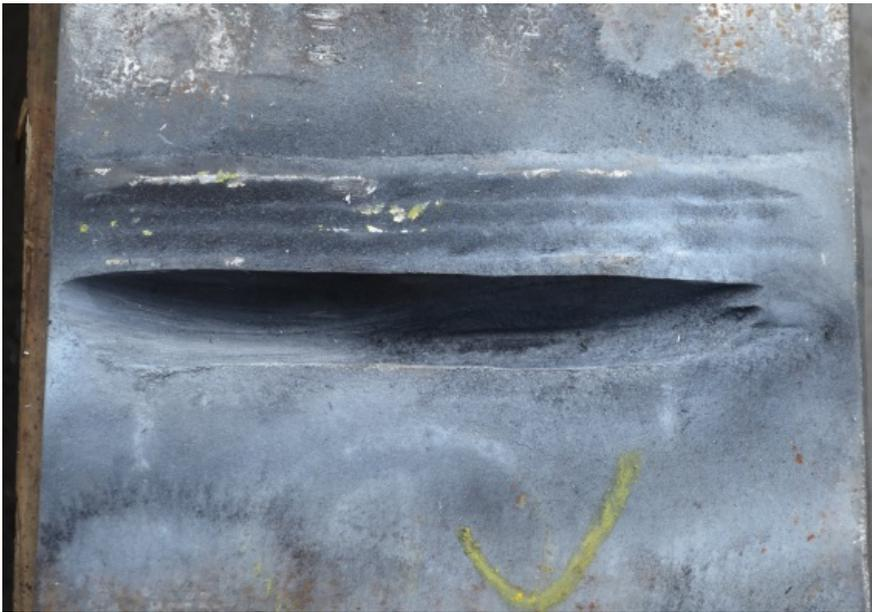
*Figure 5.17 A weld groove after crack removal process.*
