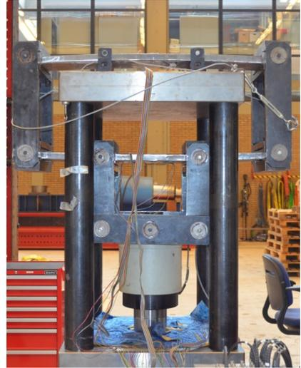
Figure 5.1 Four point bending test setup for double test specimens.
