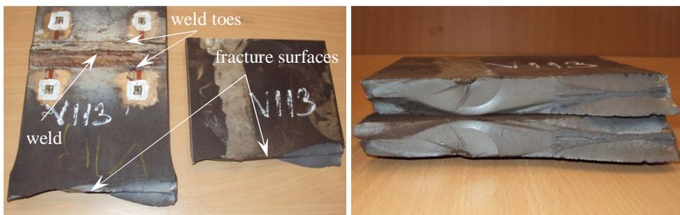
*a) Weld and crack initiation location.*
