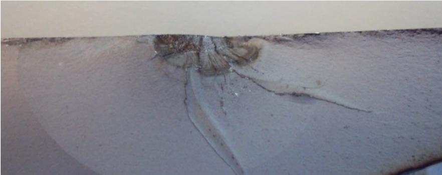
*Figure 3.13 Fatigue crack initiation location in V113 specimen.*
