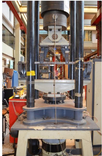
Figure 5.2 Four point bending test setup for single test specimen.
