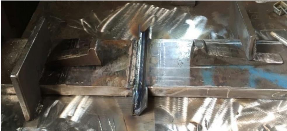
Figure 5.21 Constrained specimen during the repair weld.
