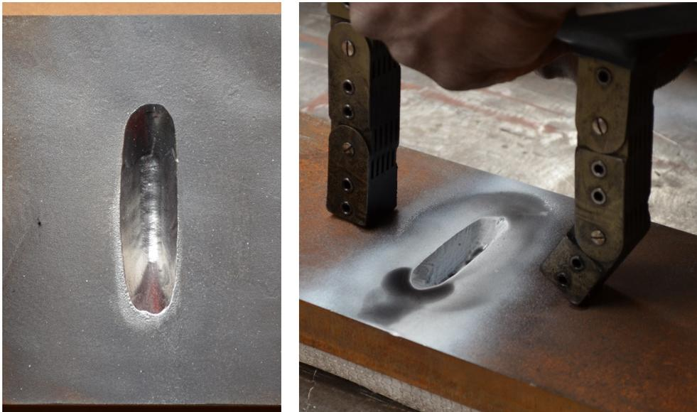
*Figure 5.12 The prepared weld groove with material removal process and NDT check on the weld groove.*
