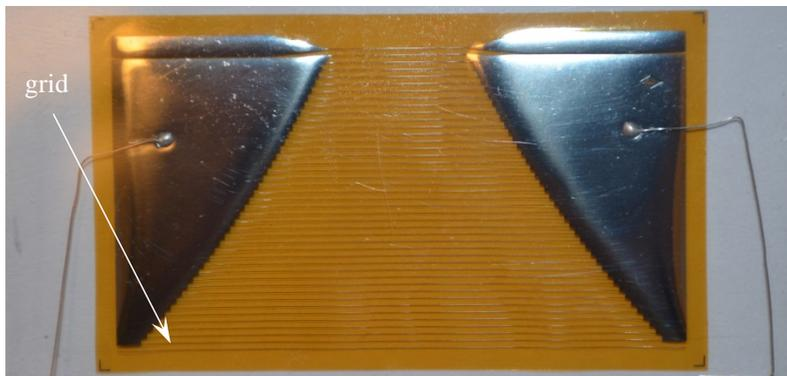
Figure 6.3 FAC-20 crack detection gauge with 41 grids.
