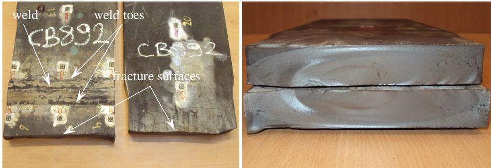
a) Weld and crack initiation location.
