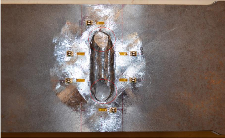
Figure 5.14 The ground start-stop point of the repair weld.
