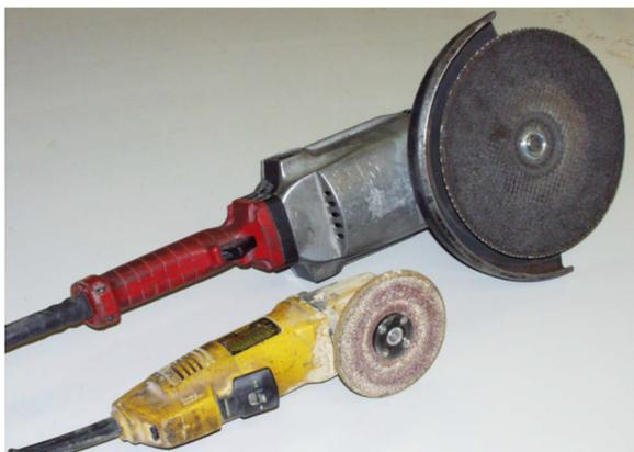
Figure 4.2 Disc grinder with different wheel size [Dexter et al., 2013].
