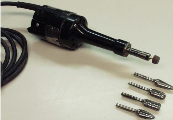
*Figure 4.4 Burr grinder with various carbide burr tips [Dexter et al., 2013].*
