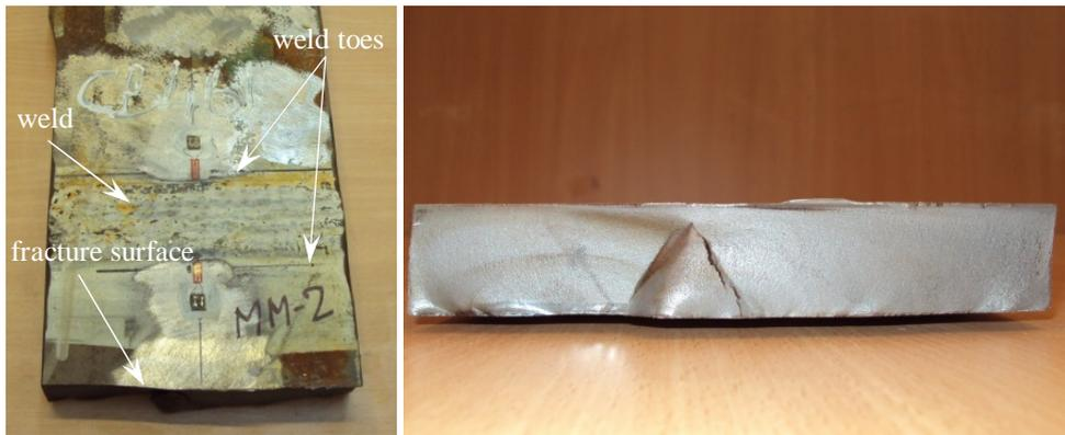
*a) Weld and crack initiation location.*
