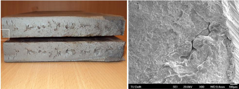
Figure 3.22 Fracture surface of C895 and imperfection at the crack initiation point.
