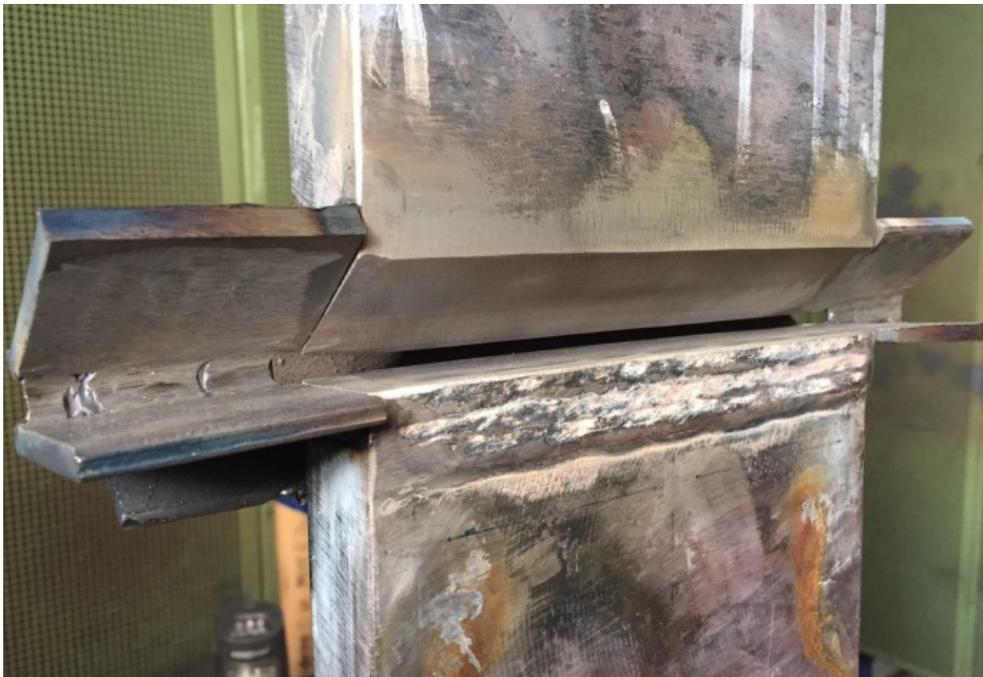
*Figure 5.20 Half V-shape weld groove and temporary plates at the edges.*
