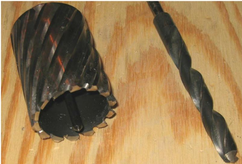
*Figure 4.13 Annular cutter and twist bits [Dexter et al., 2013].*
