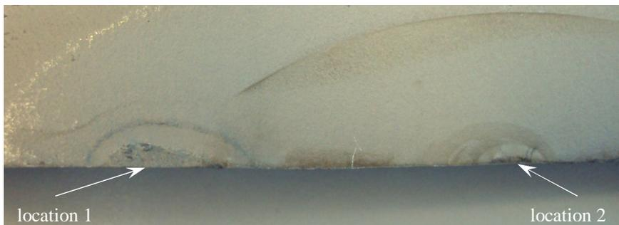
Figure 3.8 Fatigue crack initiation locations in CB892 specimen.
