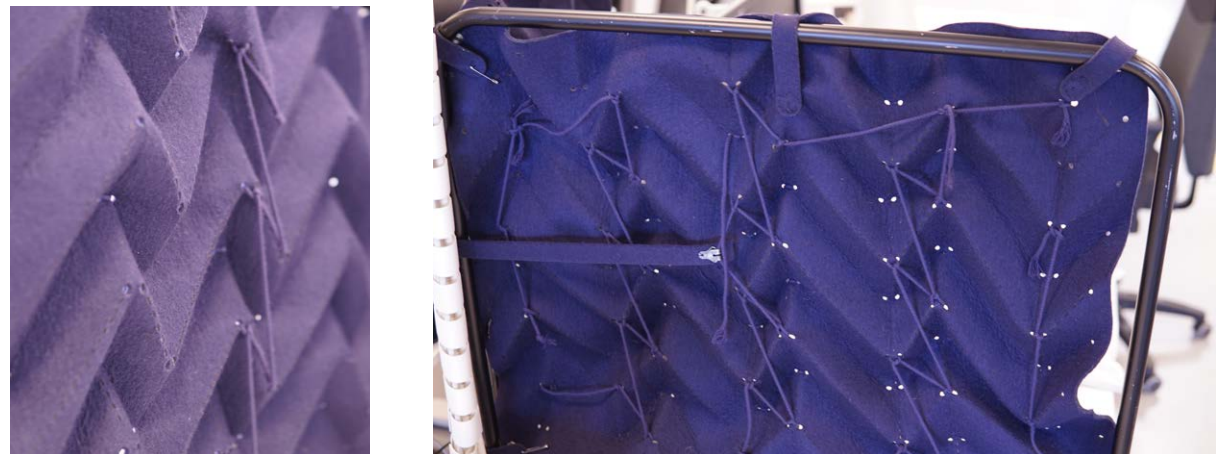
fig.47: The string at the front to prevent curving of the screen (fleft) and pattern of the knotted strings in the back (right)
