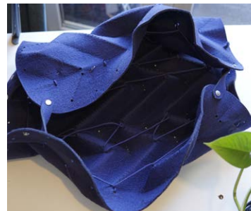
Fig.49: The buttons were unable to fold the screen compactly
