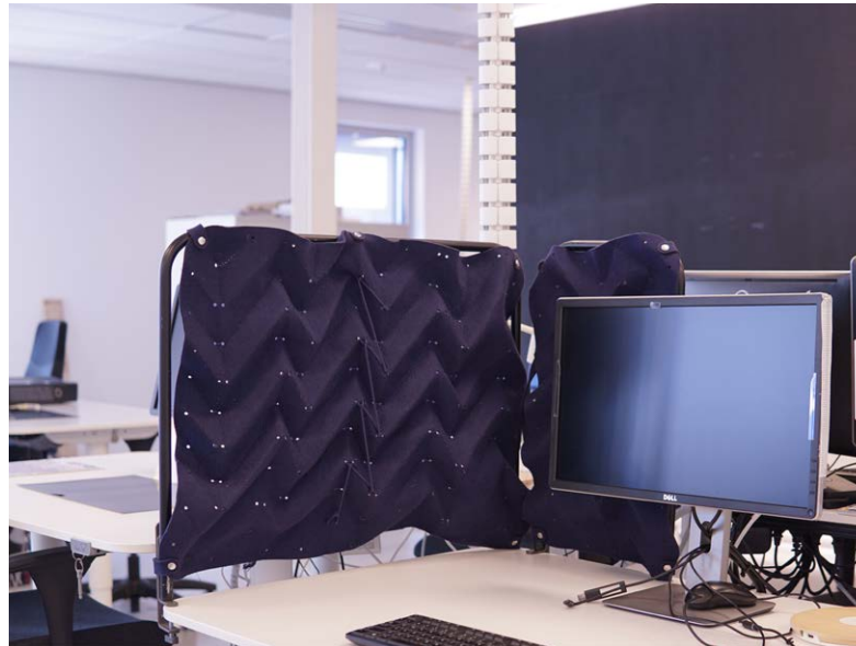
fig.52: The full scale prototype in the unfolded (left) and compactly folded (right) conditions
