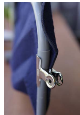
fig.53: The small-scale prototype. Left: unfolded. Middle: the paper clamps applied to attach the screen to the frame. Right: the screen in folded position
