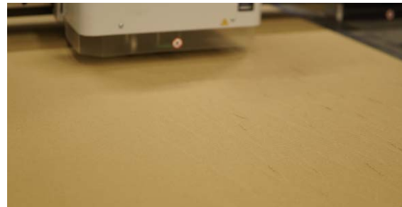
fig.40: This texture, that was cut into cardboard, could not fold compactly or repeatedly without ripping.
