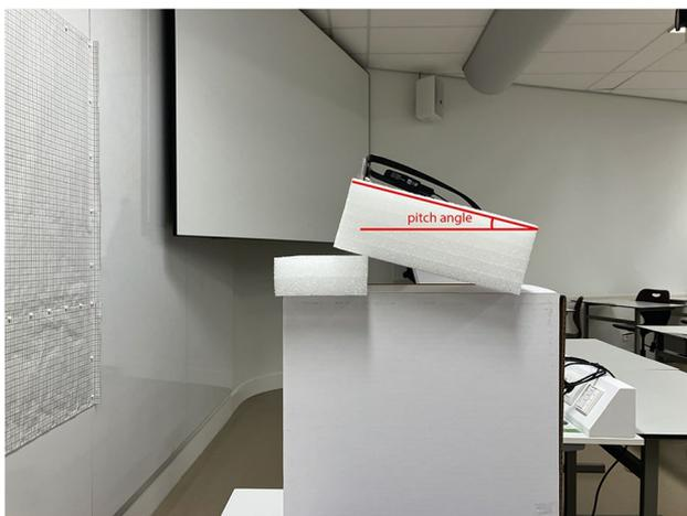
**Fig. 7** Setup for estimating the *VD* parameter. Graph paper consisting of 1×1 cm squares was stuck to the wall, and the Tobii was located at a distance of approximately 1 m from the wall
