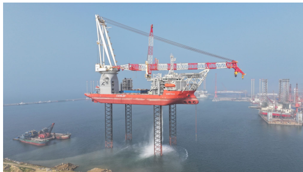
Figure 2.4: A jackup vessel. This vessel has been raised higher than necessary for demonstration purposes. Source: (OffshoreWIND.biz, 2025)
