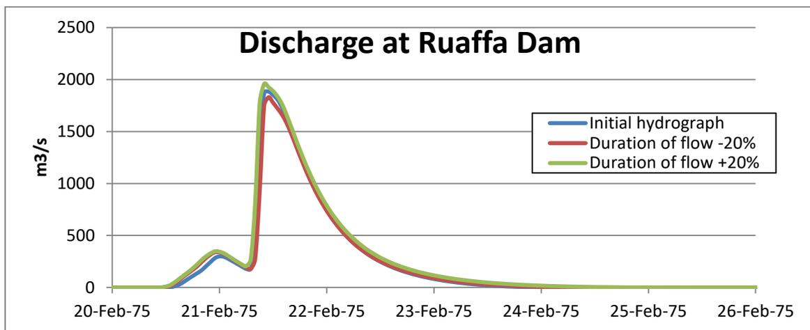
Figure L.6: Hydrograph of different duration of flow for the transmission losses
