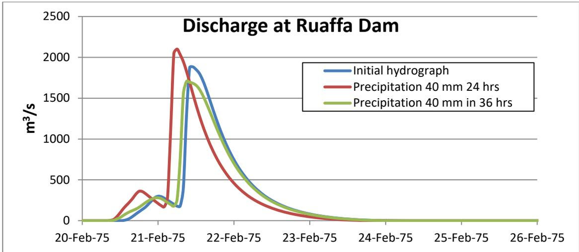
Figure L.8: Hydrograph of different precipitation duration and intensity at the Ruaffa Dam
