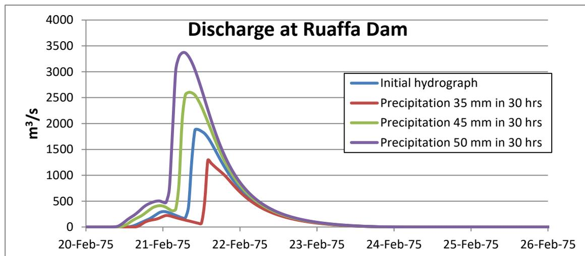
Figure L.7: Hydrograph of different precipitation amounts at the Ruaffa Dam
