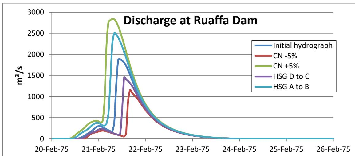
Figure L.4: Hydrograph of different CN at the Ruaffa Dam
