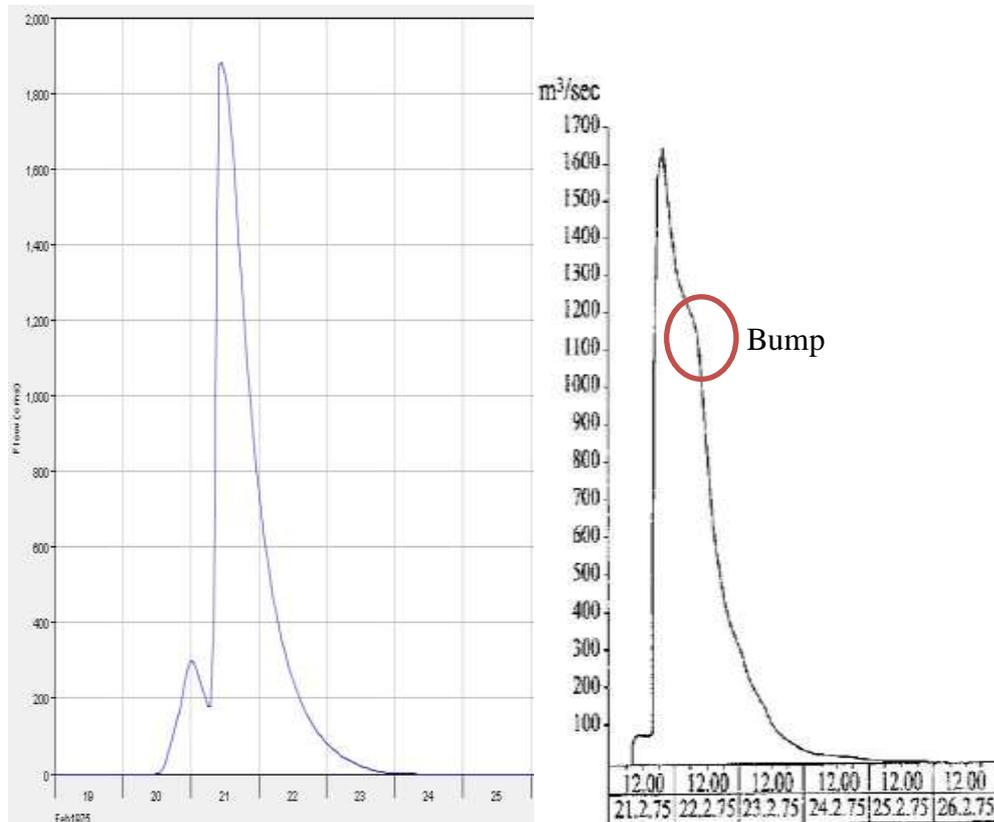
Figure K.1: Results from the HEC-HMS simulation (left) and the measured event at the Ruaffa Dam(right)
