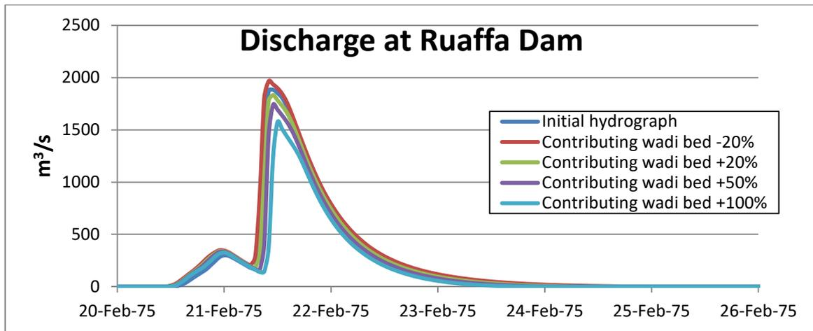
Figure L.5: Hydrograph of different contributing wadi beds for the transmission losses
