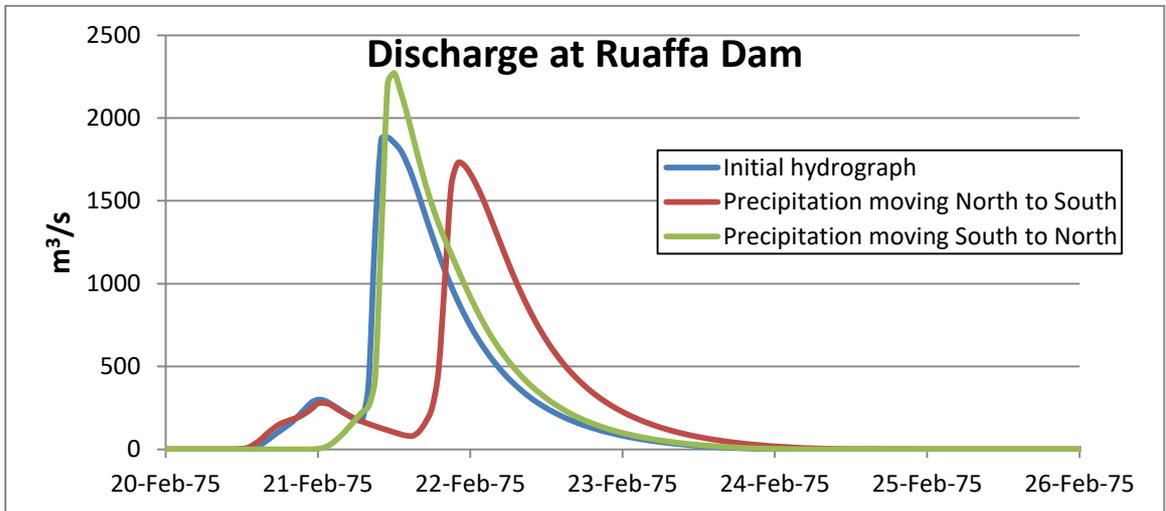
Figure L.9 Hydrograph of the effects of different storm directions at the Ruaffa Dam
