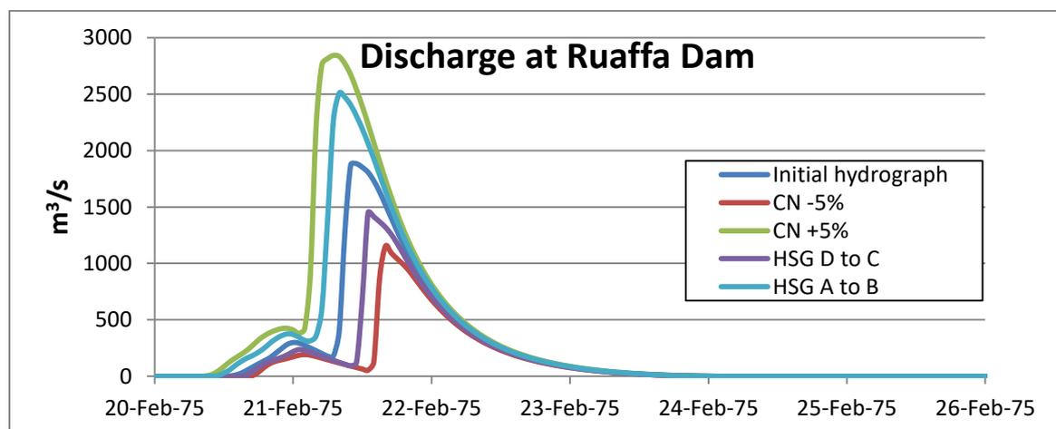
Figure 4.8: Hydrograph at the Ruaffa Dam showing the effects of the CN (own illustration, 2017)
