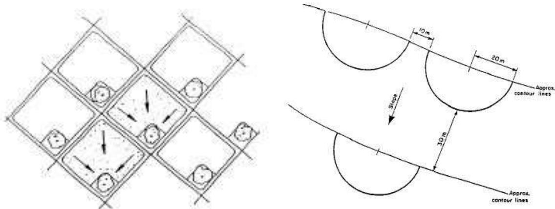
Figure N.5: Diamond shaped earthen bunds on the left (Prinz, 1996) and semi-circular bunds in the right (Critchly, Siegert, Chapman, & Finkel, 1991)
