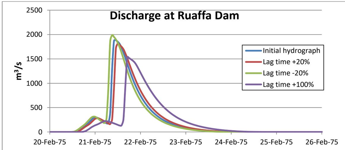
Figure L.3: Hydrograph of different lag time values
