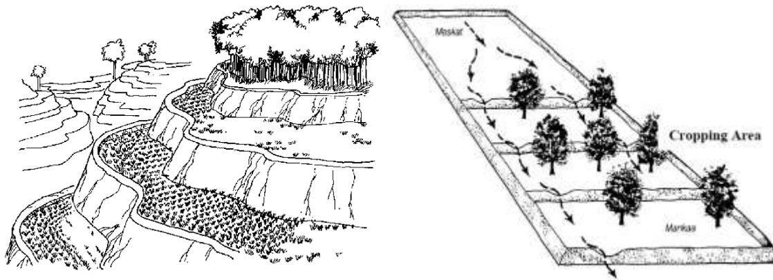
Figure N.6: Conservation bench terrace on the left (Prinz, 1996) and a Meskat system on the right (Prinz, 1996).
