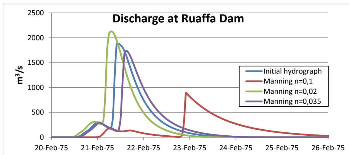
Figure L.2: The initial (0,03), lowest possible (0,02), highest possible(0,1) and adapted (0,035) Manning coefficient for natural main channels.
