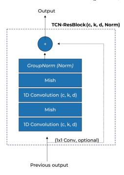
**Fig. A.1.** Structure of our TCN residual block, performing non-causal 1D convolutions with kernel size k, dilation d, and with c channels. The final group normalization is optional when *Norm* is set. Based on [46].
