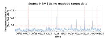
**Fig. 9.** Anomaly scores of the target WT test set. The reconstruction errors are obtained from the pretrained source WT NBM using the mapped target test set data.
