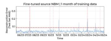
Fig. 8. Anomaly scores of the target WT test set from the fine-tuned source NBM using scarce target training data.
