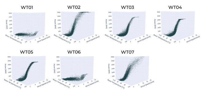
Fig. A.2. Scatter plots of the mean power, wind speed, and rotor temperature of a subset from filtered training samples illustrating the differences across all 7 WTs used in our experiments.
