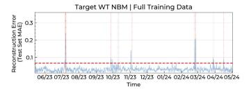
**Fig. 6.** Anomaly scores, i.e., reconstruction errors, of the target WT test set obtained from the representative NBM. The model-specific threshold is shown as a red dotted line, while time frames with logged incidents are marked by red shaded areas.
