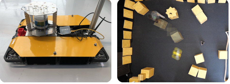
Figure 7.5: Real ground robot used to run the experiments. For the real-world experiment, we used a Clearpath Dingo with a Velodyne VLP16 mounted on top (left). The real-world experiment shows the Dingo navigating through an environment where a human throws in obstacles (right).
