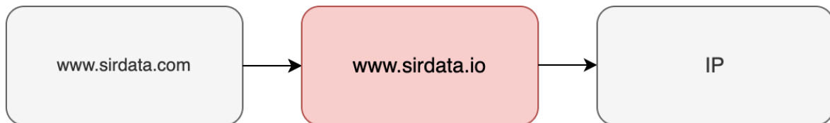
Figure 6.20: DNS resolution of www.sirdata.com .
