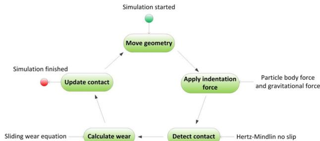
Figure 3. Simulation cycle of a pin-on-disc wear test
