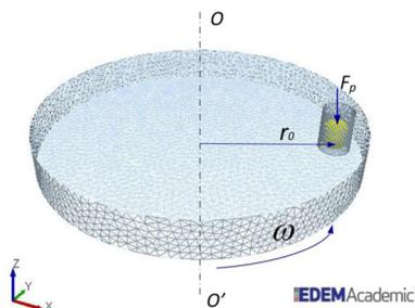
**Figure 2.** Pin-on-disc simulation model
