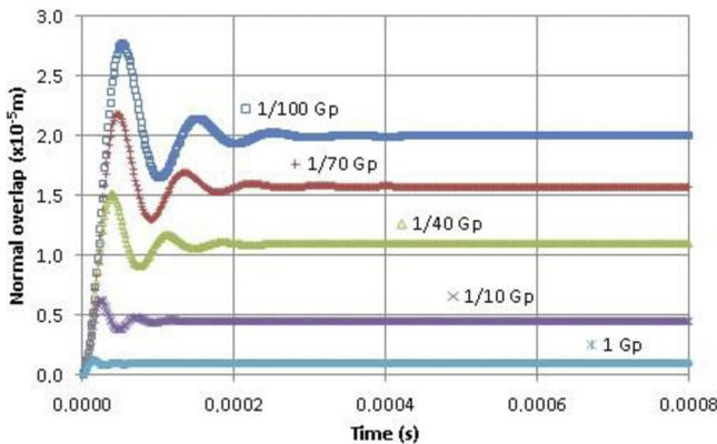
**Figure 16.** Normal overlaps as functions of particle shear moduli
