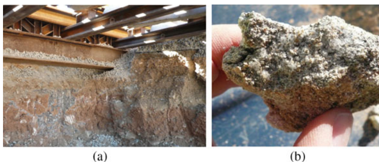
Fig. 13 a Upper meters of the compacted fill of one of the embankments. Exposed surface excavated during the underpinning works; b detail of a cement-soil mixture found at the cut surface
