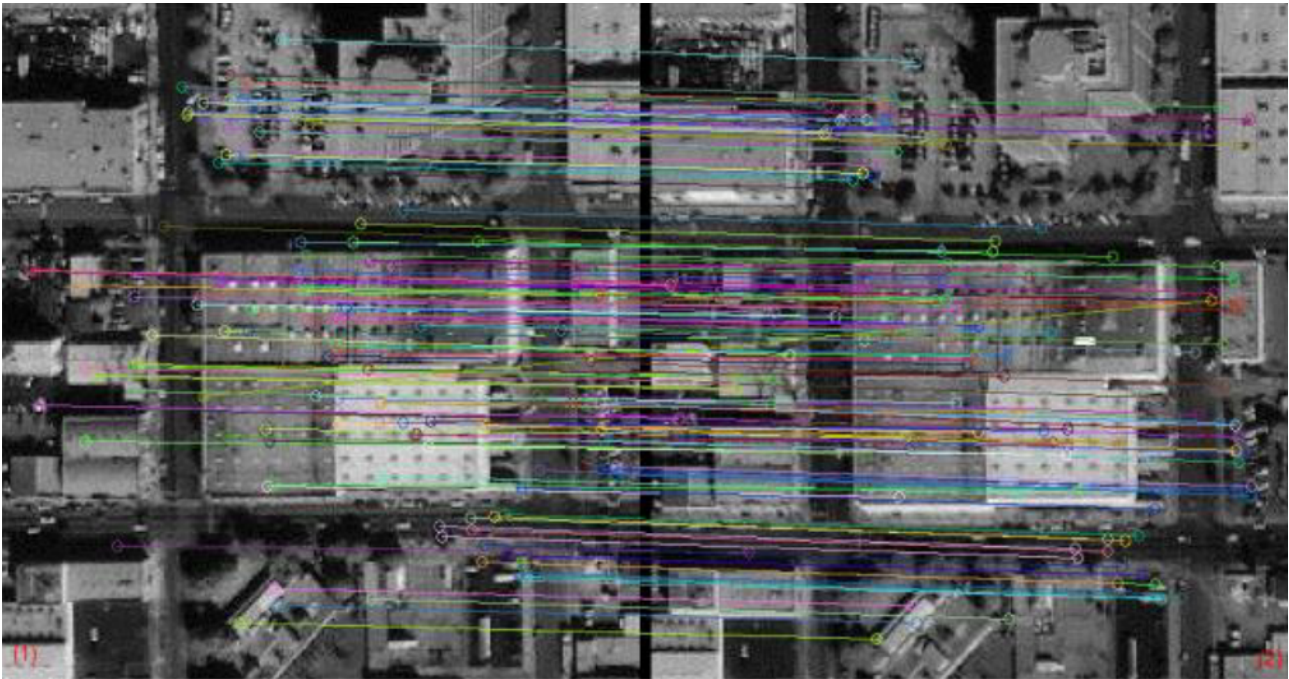
Figure 2.8: Example of GCP tie-points between two similar images [34]. Note how the matched features are predominantly permanent structures that exist in both images.
