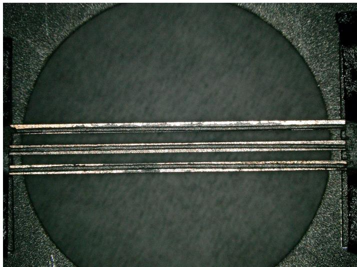
Figure 3.4: An image by the optical microscope of the auxiliary coil. The wires are coated with conducting silver paint to hide the insulating material from the electron beam.
