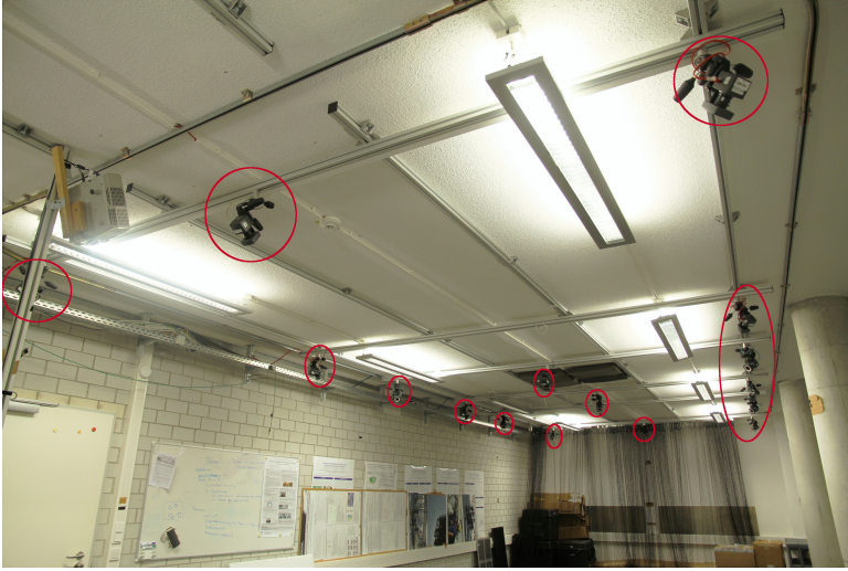
Figure 5.1: The Holodeck at the DLR premises. The circles highlight the VICON camera system, which is used for indoor positioning and motion tracking.
