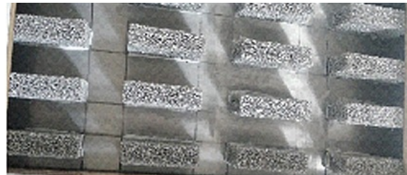
Figure 14: Impression of the porous aluminium fins configuration on the test section. Image taken from Bilen et al., 2017.
