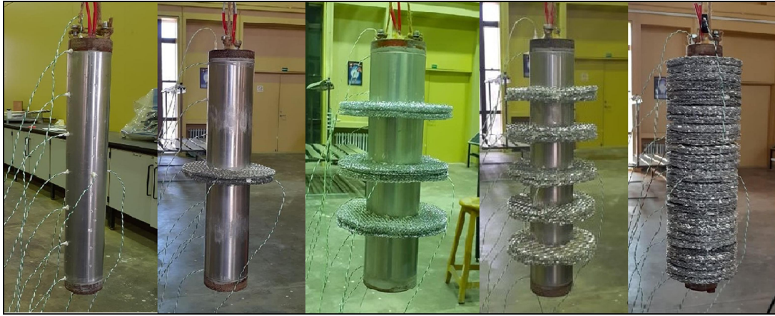
Figure 20: Some examples of the annular porous fins attached to a suspended heated cylinder that were tested by Kiwan, Alwan, and Abdelal, 2020.
