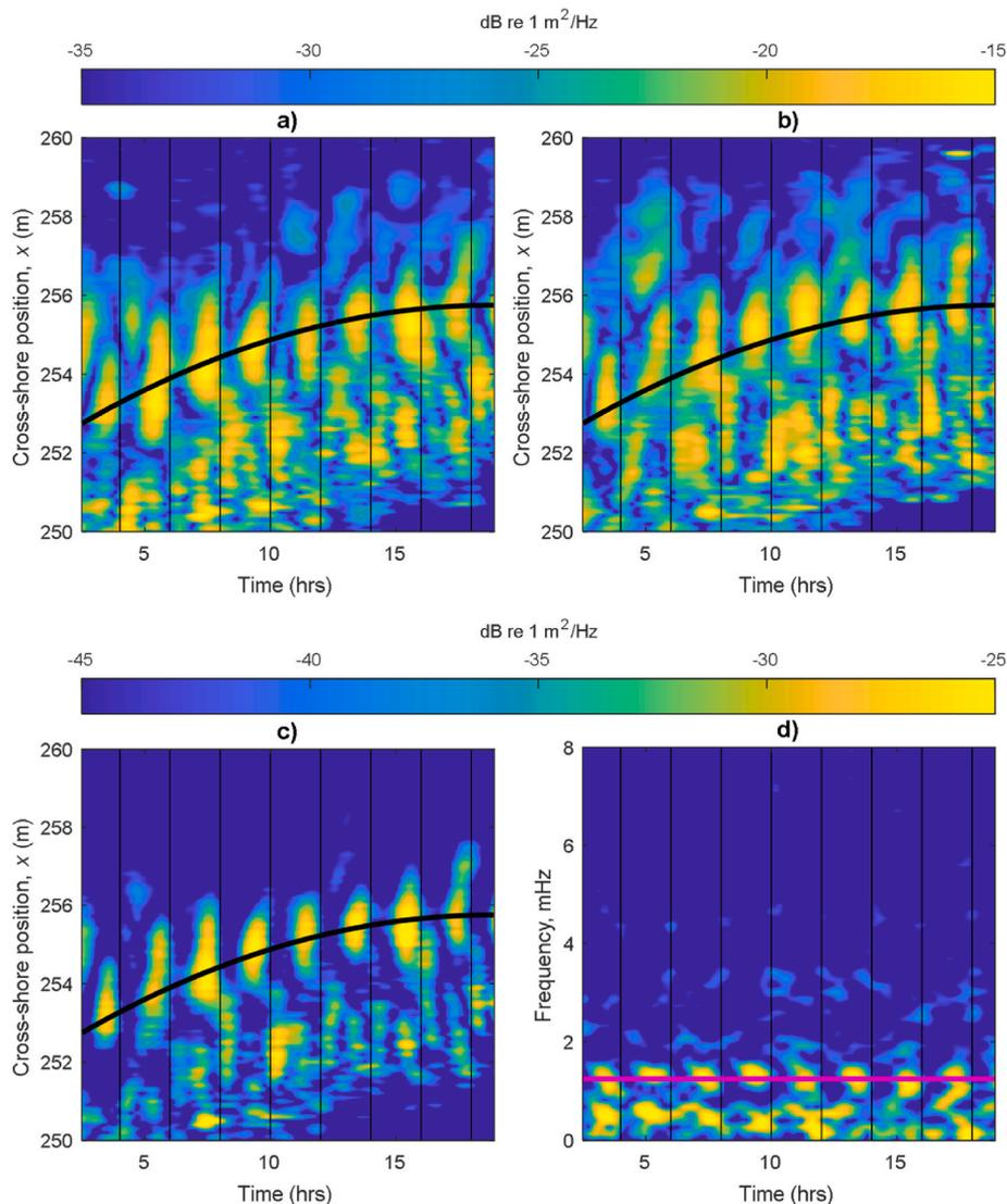
**Fig. 8.** Top row) Spatial distribution of spectral power at 1.25 mHz as a function of time for a) Experiment SB, and b) Experiment DR. Bottom row: c) Cross-spectrogram between Experiments SB and DR, and d) cross-spectrum extracted along the thick black line in panel c which follows the peaks in spectral power. The horizontal pink line indicates  $f = 1.25 \text{ mHz}$ . The vertical black lines in all panels indicate the start of each 2-h wave signal repeat.
