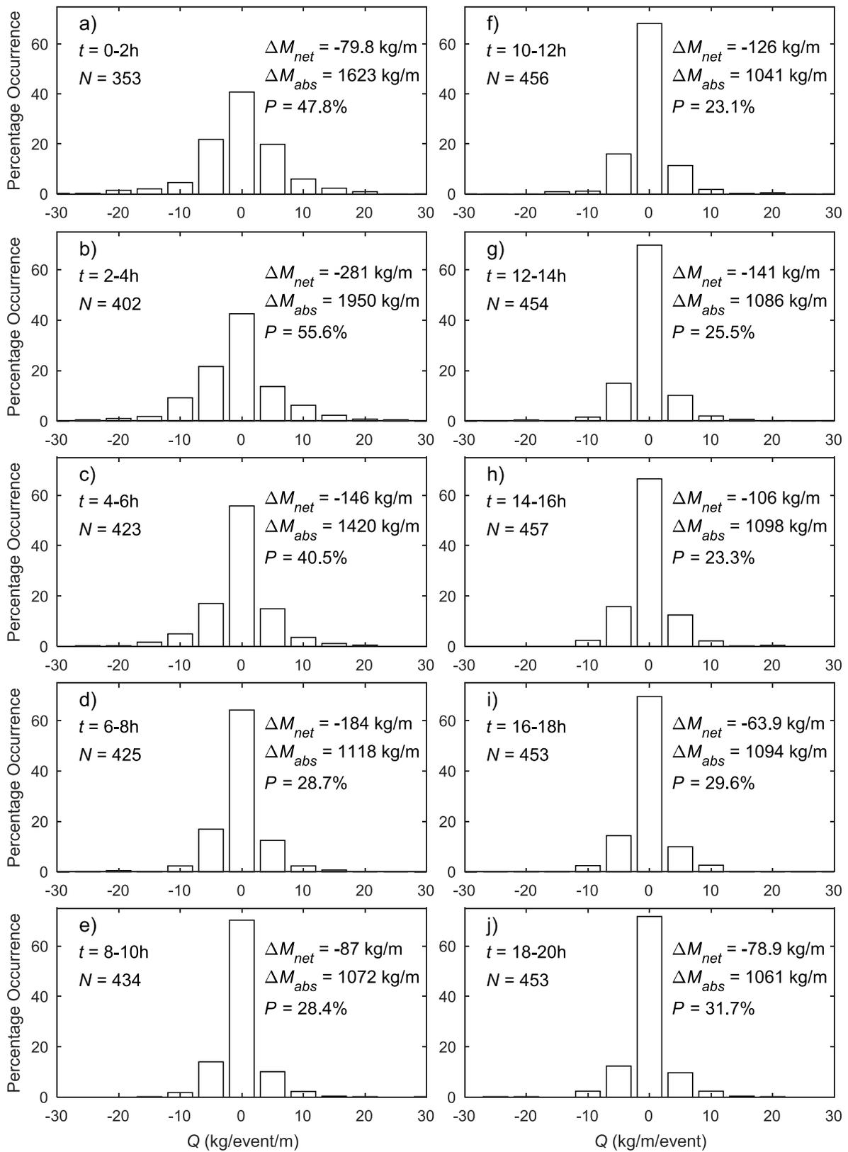
**Fig. 10.** (a to f) Histograms of the cross-shore net mass flux due to every detected swash event at a constant relative position in the swash zone ( $s_{120} = 29\%$ ) during each 2-h repeat of the wave signal for Experiment SB.  $s_{120} = 29\%$  corresponds to  $x = 254.3$  m during the first 2-hour period. N indicates the number of swash events detected and P is the percentage of gross volume change caused by single event fluxes larger than  $\pm 7.5$  kg/m/event.
