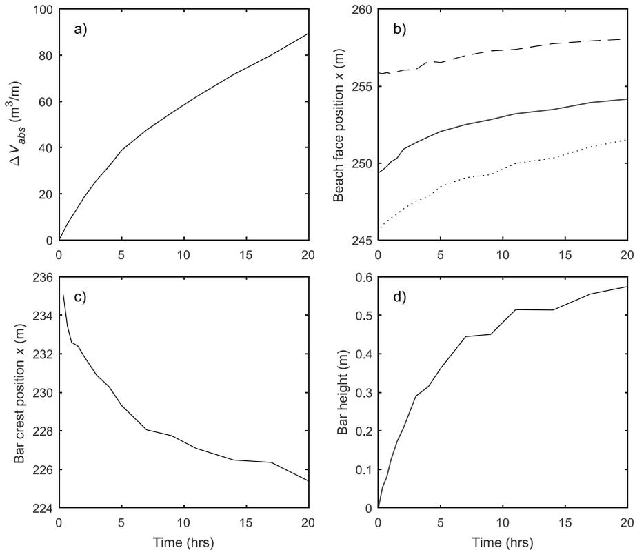
Fig. 2. Temporal evolution of morphological indicators obtained from the mechanical profiler measurements during experiment SB: (a) cumulative absolute change in beach volume landward of  $x = 200 \text{ m}$ . (b) Horizontal position of 3 characteristic points on the beachface: solid line = SWL; dashed line =  $R_{2\%}$ ; dotted line = 2% rundown limit. (c) Cross-shore position of the primary bar crest. (d) Primary bar height measured relative to the initial planar profile.
