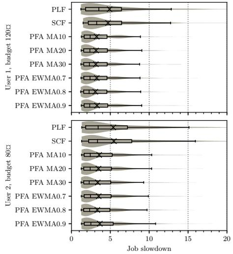
Figure 5.6: Variability of job slowdowns for all the studied autoscalers with different budgets for each user when running WL I. PFA autoscaler was executed with different smoothing methods. Means are marked with  $\times$ .
