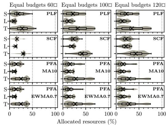
Figure 5.14: Variability of allocated resources for User 1 for the studied autoscalers with equal budgets of 60, 100, 120 when running WL I. For Small and Large resource types, and in Total. Means are marked with  $\times$ .
