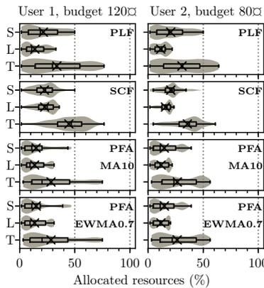
Figure 5.15: Variability of allocated resources for each user with different budgets 120 and 80 when running WL I. For Small and Large resource types, and in Total. Means are marked with  $\times$ .
