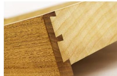
Figure 43: Dovetail joint
