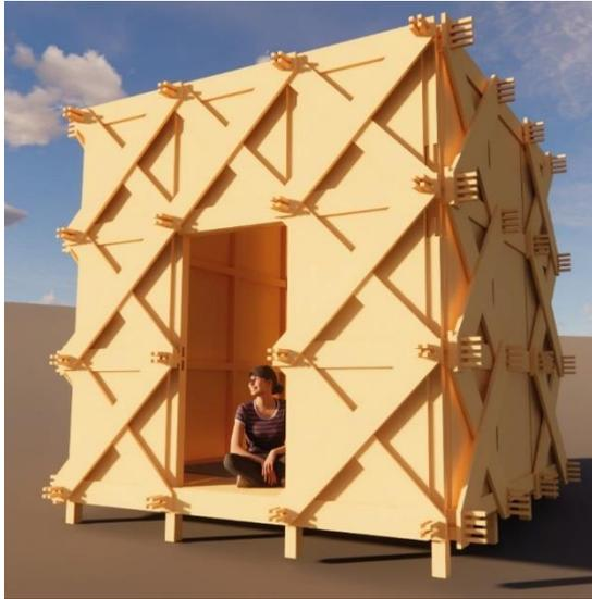
Figure 25: Tsugite shelter design of a 3 by 3 unit
