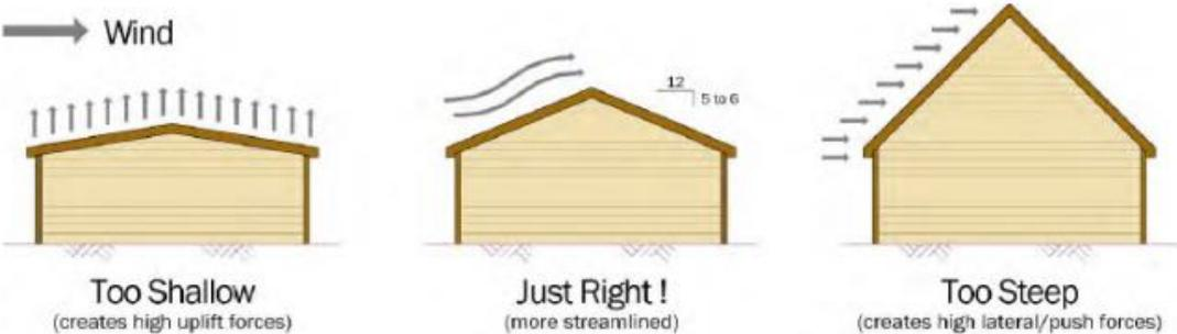
Figure 75: Optimal roof pitch
