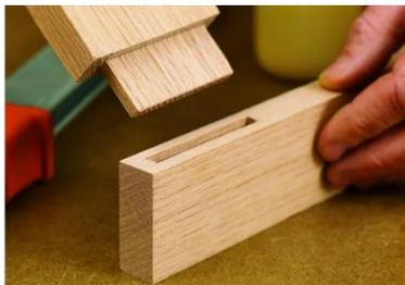
Figure 43: Mortise and tenon joint
