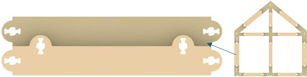
Figure 140: Element that joins two frames together
