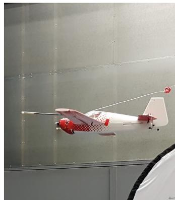
Figure 5.1: Slick 360 Micro model with autopilot and sensors
