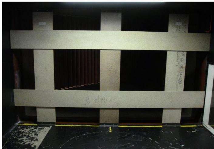
Figure 2.7: Turbulence grid set-up at test section inlet [25]
