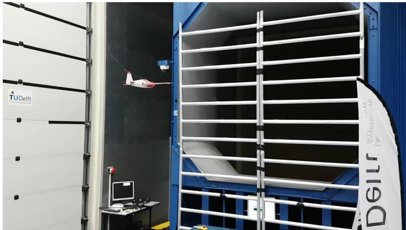
Figure 5.7: Turbulence grids set-up
