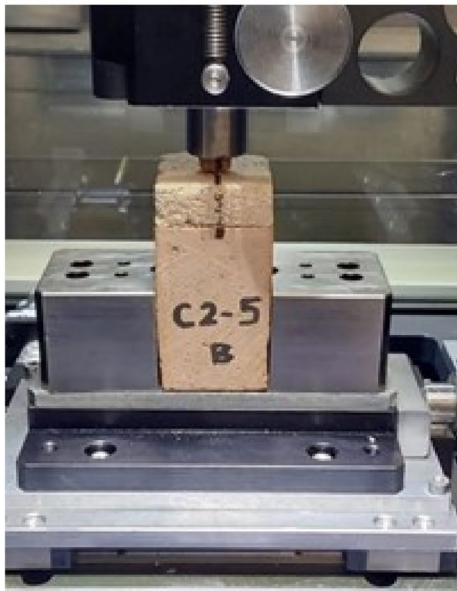
Fig. 1 Reciprocating tribometer setup and specimen with cracked brick-mortar interface
