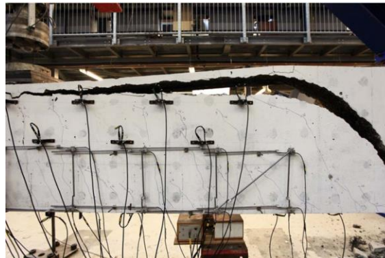
Figure 3.3 Typical LVDT's array
