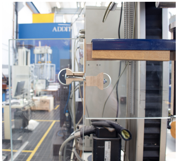
Images for step 6 after reaching to the ultimate point and failure in connectors
