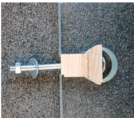
Figure 8.3.58 ,63, Deliberate overload applied to reveal ultimate failure characteristics of the joint. Source: Author's own.
