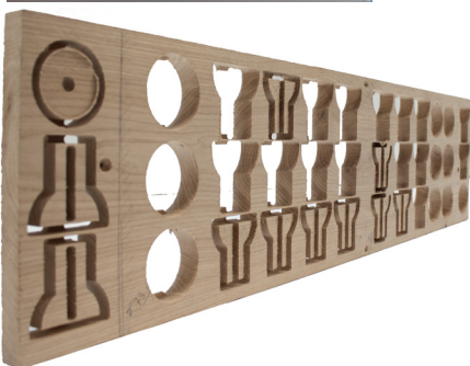
Figure 8.3.42 to 46, Final Glass test prototype, Sedak sticker on glass, Oak used for CNC milling connector, Oak timber after CNC cut geometries came out. Source: Author's own.
