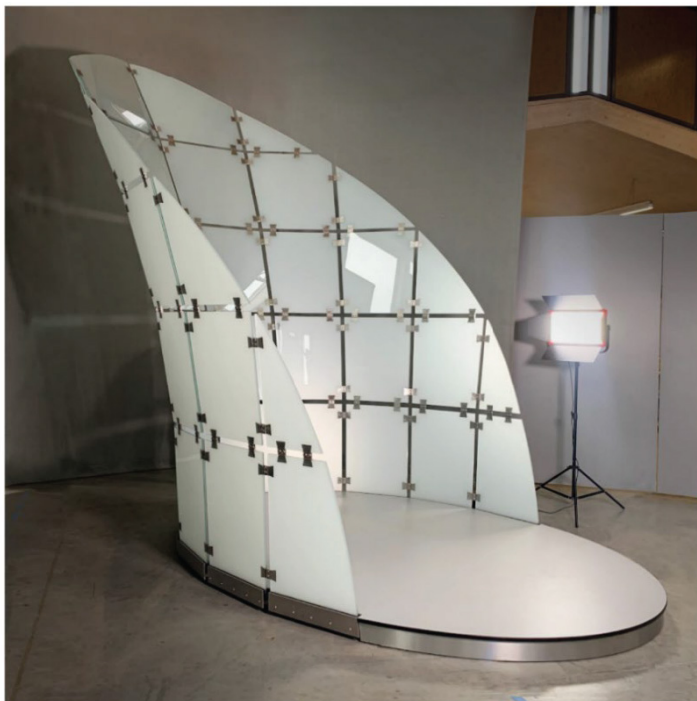
Figure 68: Photography of the assembled frameless glass structure. Source: Stevels, W., Fildhuth, T., Wüest, T., Haller, M., & Schieber, R. (2022). Design Base for a Frameless Glass Structure Using Structural PVB Interlayers and Stainless-Steel Fittings. Challenging Glass Conference Proceedings, 8, 369. https://doi.org/10.47982/cgc.8.369
