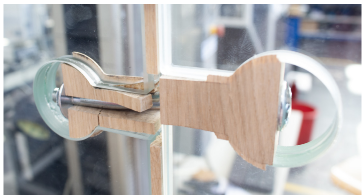
Figure 8.3.58 ,63, Deliberate overload applied to reveal ultimate failure characteristics of the joint. Source: Author's own.
