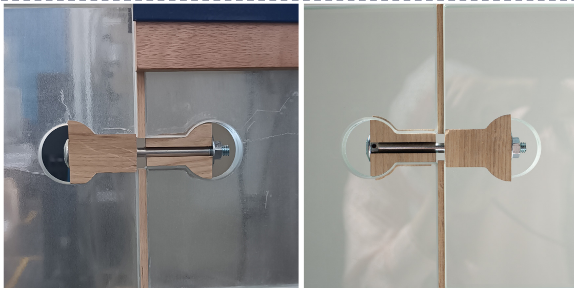
Figure 8.3.78 & 79, left, perpendicular to grain direction in loading position, Right parallel to grain direction in loading position. Source: Author's own.
