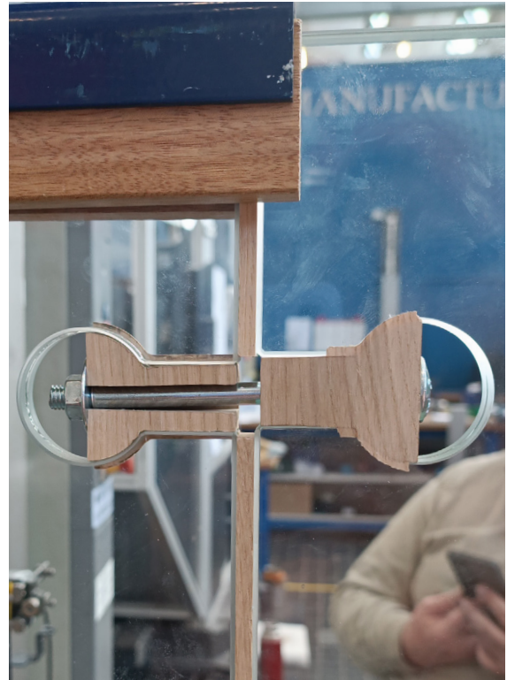
Images for step 6 after reaching to the ultimate point and failure in connectors
