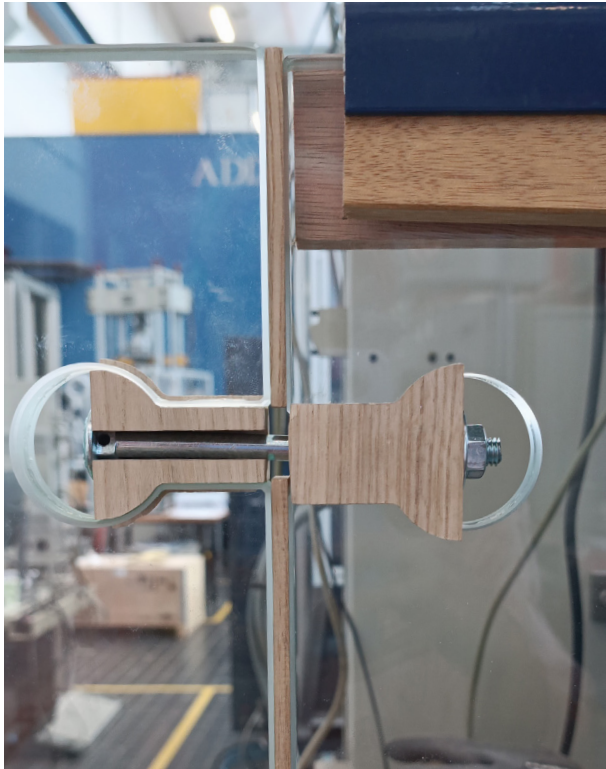
Images for step 6 after reaching to the ultimate point and failure in connectors
