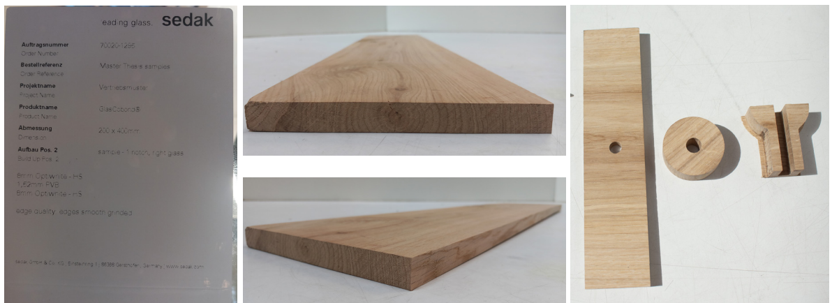
Figure 8.3.42 to 46, Final Glass test prototype, Sedak sticker on glass, Oak used for CNC milling connector, Oak timber after CNC cut geometries came out. Source: Author's own.
