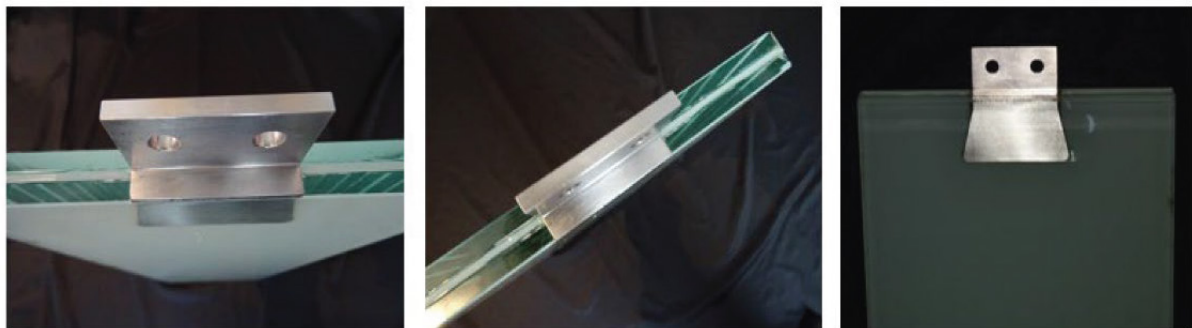
Figure 70: Different views of the laminated Ptting: top view at angle (left), top view perpendicular (center) and side view (right) for specimen with Ptting on short edge.
