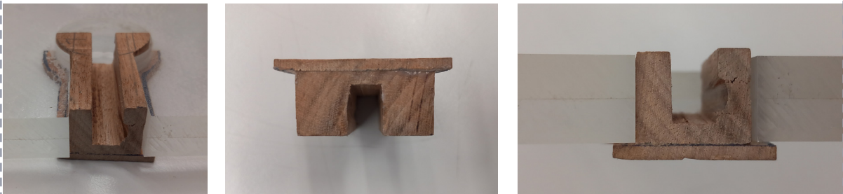
Figure 8.3.33 to 35, Pre-test prototype, Deformation in wooden components. Source: Author's own.
