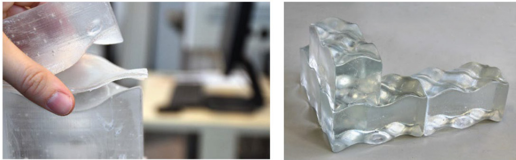
Figure 78: Left: Typical Y breaking pattern, originating at the shortest section of the block during test under static load of 40 kN (14.2 MPa) by (Oikonomopoulou, 2019). Right: Possible explanation of the cause of failure of the specimens interleaved with PMC770 (70A) and Task16 (80A). Derived from (Oikonomopoulou, 2019b)
