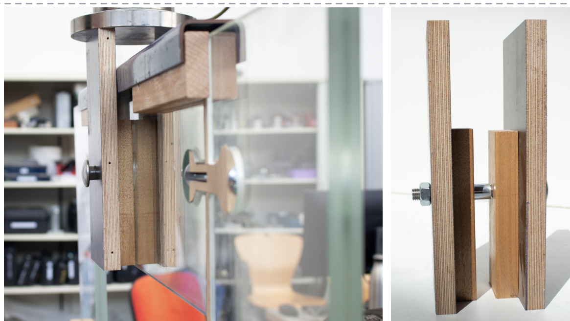
Figure 8.3.51, Revision in applying point load, bigger bolt M12, rivet, and wooden clamping surface. Source: Author's own.
