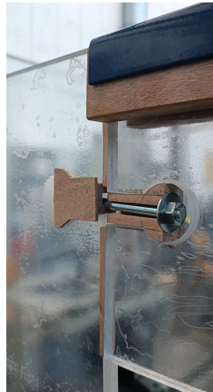
Figure 8.3.36, Pre-test prototype, Bolt deviation due to exceeding preload in joint in loading until failure scenario Source: Author's own.
