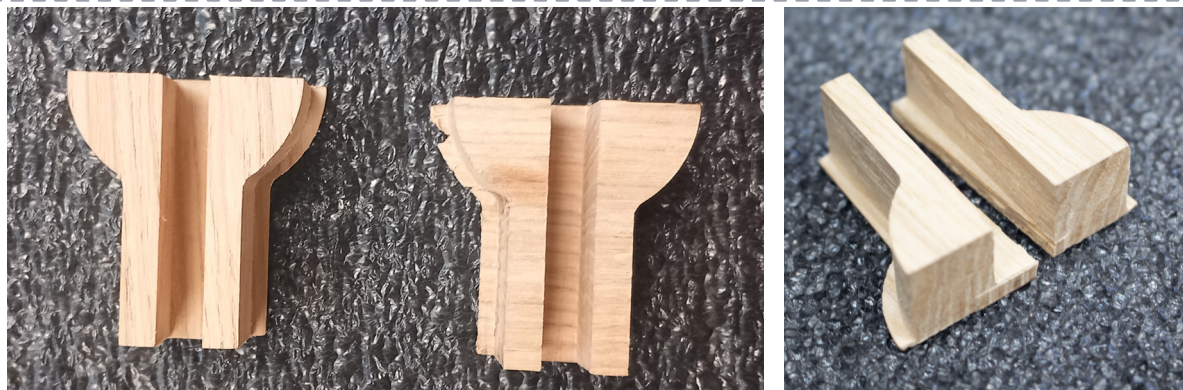
Figure 8.3.77, left, perpendicular to grain direction in loading position, Right parallel to grain direction in loading position, far right, if applied torque is done fast and with out system of pin driver, most likely the square neck of bolt will rotate and break the wood specially in this direction was fragile than then other one. Source: Author's own.
