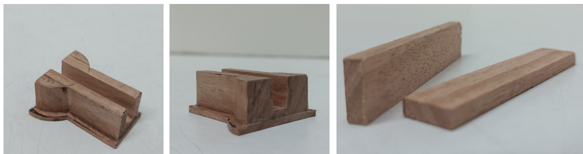
Figure 8.3.1 to 3, Pre-test prototype, Meranti wood Connector and spacers. Source: Author's own.
