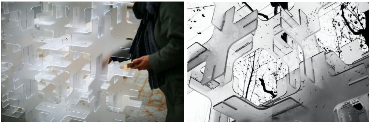
Figure 46: Close view of modules, made of recycled offcuts of commercial polycarbonate sheeting "Temporary Permanence Installation" by Arup Associates, Source: ArchDaily. (2016).
