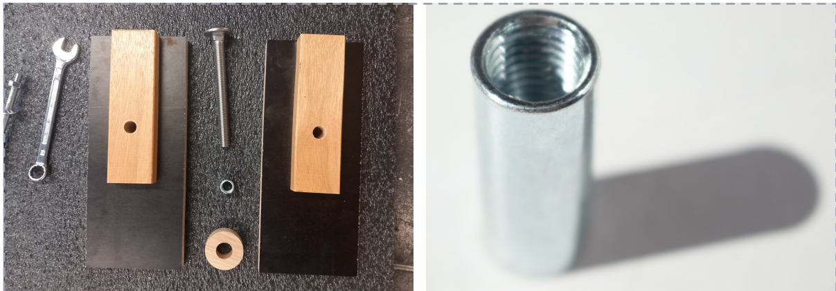
Figure 8.3.52, Revision in applying point load, bigger bolt M12, rivet, and wooden clamping surface. Source: Author's own.
