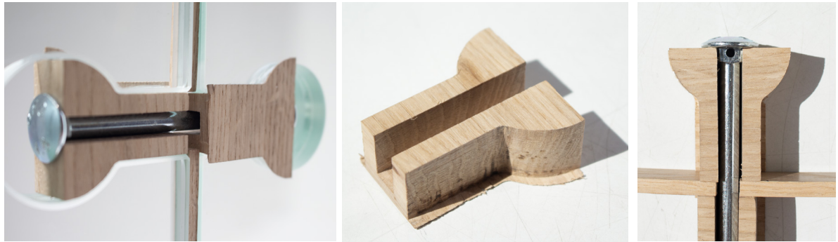
Figure 8.3.50, rectangular groove to fit the square neck bolt better. Source: Author's own.
