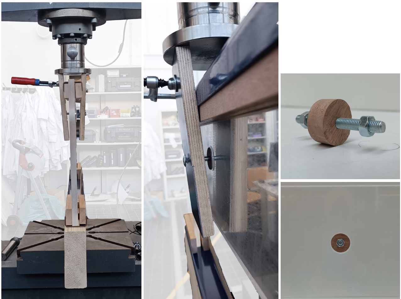
Figure 8.3.14 to 17, Pre-test prototype, Point load lab set ups. Source: Author's own.
