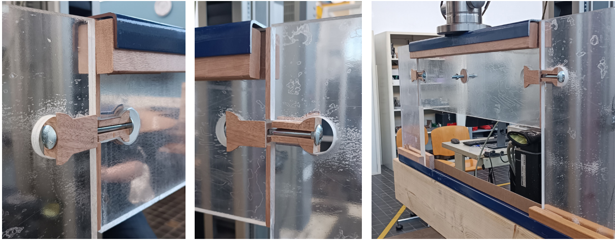
Figure 8.3.9 to 11, Pre-test prototype, UDL loading results after 10 minutes. Source: Author's own.
