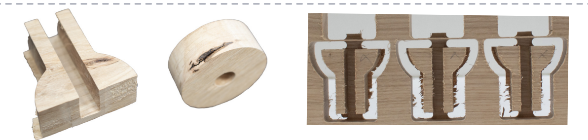
Figure 8.3.49, Natural imperfections in wood and some errors during fabrication. Source: Author's own.
