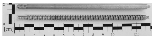
Figure 5. Model of the straight shafted pile and the screw-type pile; both piles had an embedment length L_0 \approx 90 mm
