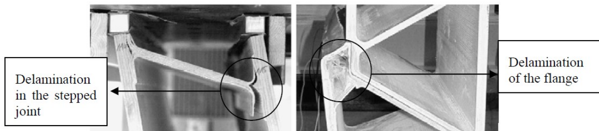
Figure 2-31 Failure modes of Duraspan in the left and ASSET deck in the right for in-plane compression tests (Keller & Gürtler, 2006)
