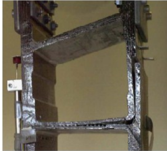
Figure 2-33 Failure in the joint for in-plane tension test in Duraspan deck (Keller & Schollmayer, 2006)
