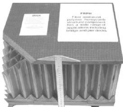
Figure 2-16 Honeycomb sandwich configuration (NCHRP, 2006)
