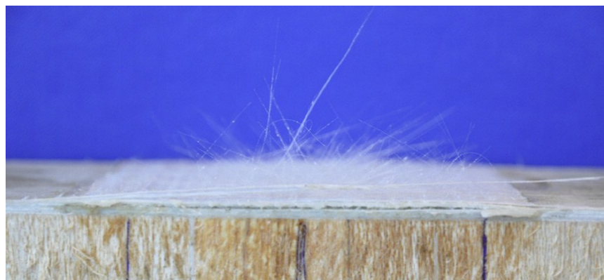
Figure 2-38 Delamination failure of SP-specimen01 (Jiang, Kolstein, & Bijlaard, 2013)
