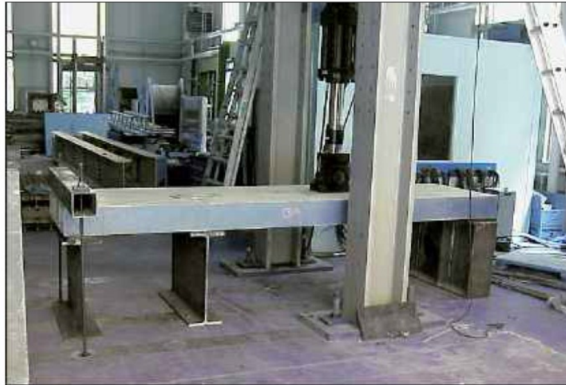
Figure 2-55 Global fatigue specimen (Cassity, Richards, & Gillispie, 2002)
