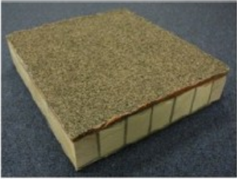
Figure 3-6 Ecosafe deck (Jiang, Kolstein, & Bijlaard, 2013)
