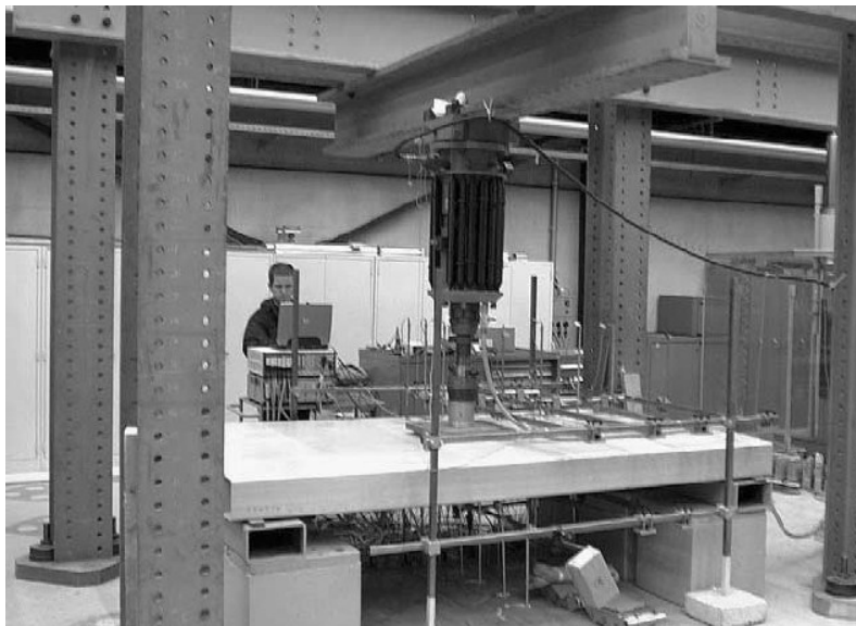
Figure 2-34 Experimental set-up for static tests performed by (Keller & Schollmayer, 2004)
