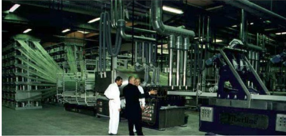
Figure 2-11 Fiberline Pultrusion Equipment (NCHRP, 2006)
