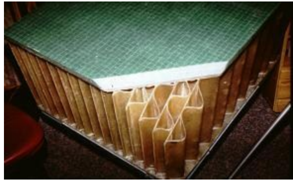
Figure 2-10 Kansas Structural Composites Honeycomb Deck Section (FHWA, n.d.)
