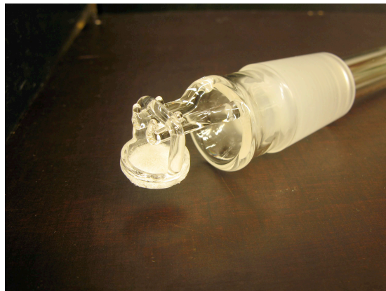
Figure 62: Single particle furnace at Åbo Akademi University and particular of the quartz sample holder
