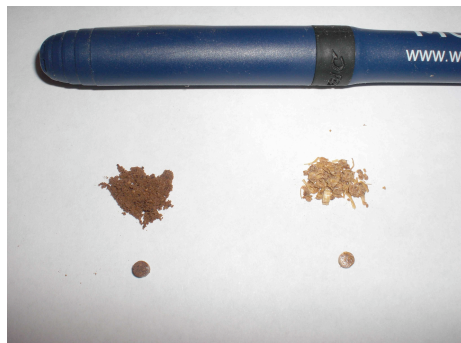
Figure 52: Samples of PKC and DDGS as used in the heated foil reactor
