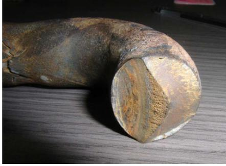
FIGURE 2.9: Fatigue fracture surface of a chain link
