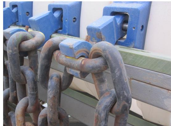
FIGURE 2.6: Chain link 30x108 mm and plastic attachment
