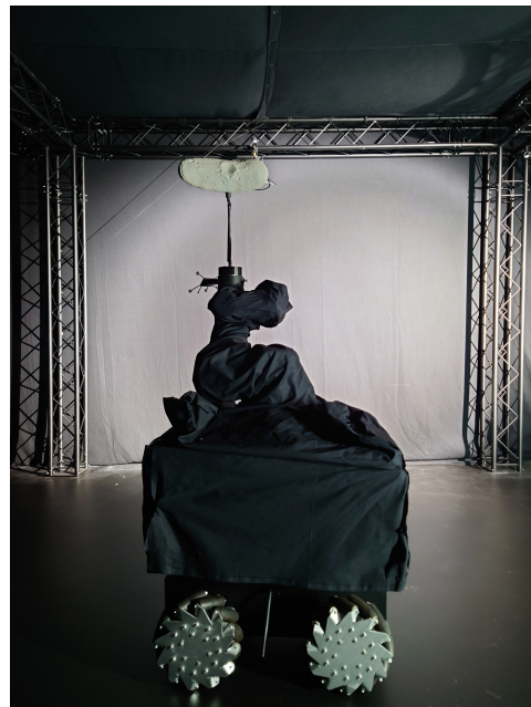
(b) Robot 1: RB-Kairos rover base with a UR16e robotic arm oriented with the tool flange is parallel to the ground, enabling attachment of a 3D-printed asteroid model.
