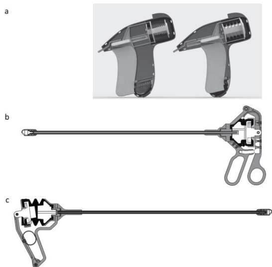
Figure A1.2. A1.2a) The first handle design based on ergonomic guidelines ( Project Advanced Products, ....., I Sorgendal ), A1.2b) The second handle design based on a conventional laparoscopic mechanical grasper, and A1.2c) The third handle design which was design according the philosophy of ‘form follows function’.
